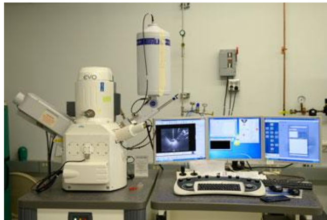
Figure 3.8 Scanning Electron Microscope model ZEISS EVO 50
