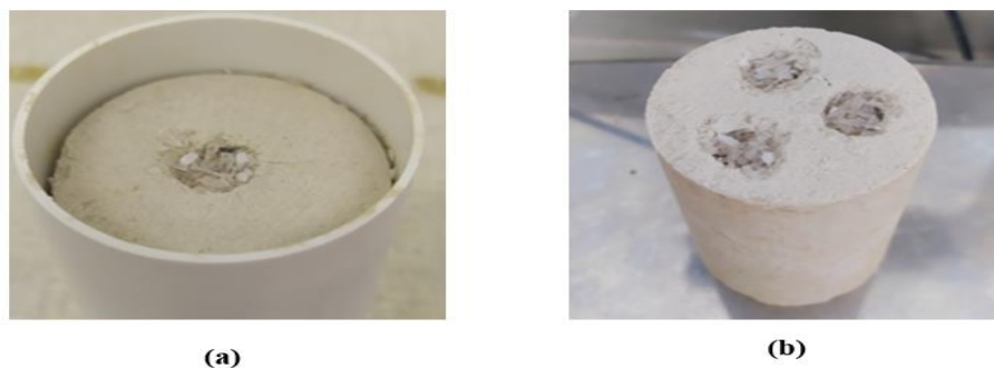
Figure 3.14 Reinforced kaolin sample with PET (a) Single PET column (b) Group PET columns
