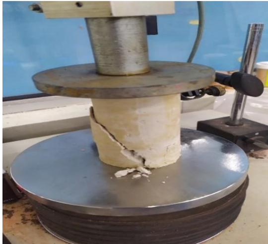
Figure 3.9 Unconfined compression test (UCT) on kaolin specimen
