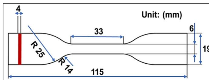
**Fig. 1.** Specifications for the size and shape of tensile test specimens
