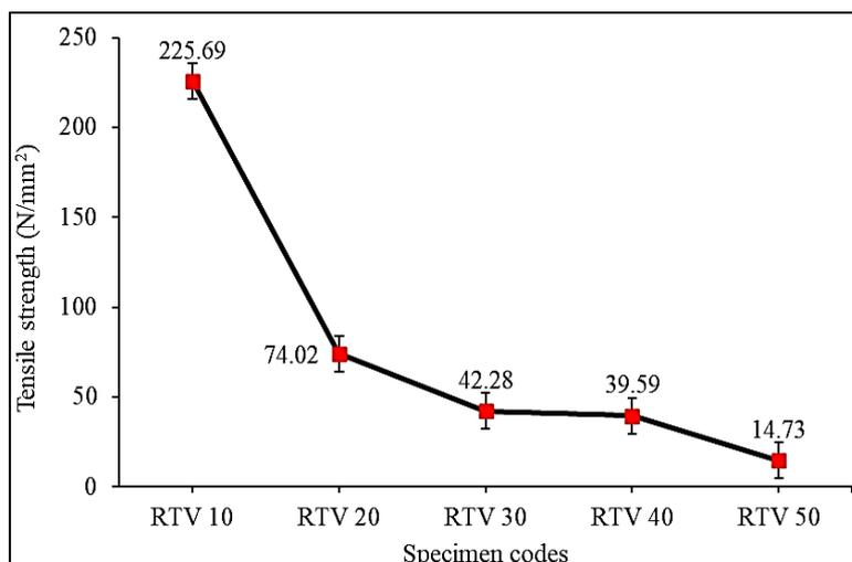
**Fig. 4.** The effects of filler additions on the composite specimen's tensile strength
