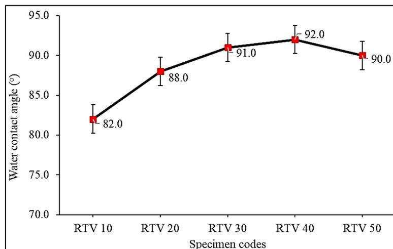
**Fig. 2.** The effects of filler additions on the composite specimen's water contact angle
