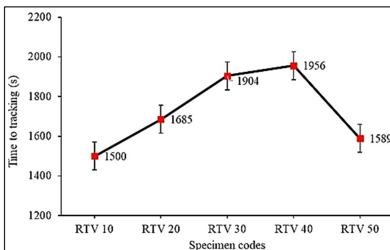
**Fig. 3.** The effects of filler additions on the composite specimen's time to tracking
