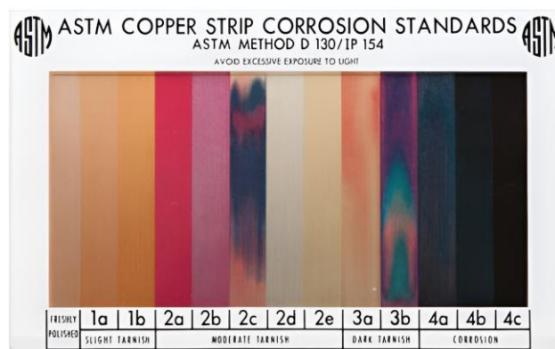
Figure 8 Classification of Copper Strip Corrosion Standards According to ASTM D4048
