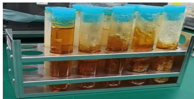
Figure 7 The immersion of copper strips into test tubes of greases before being heated into hot water and oven
