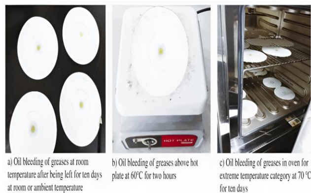
Figure 4: Oil bleeding analysis at three different types of conditions
