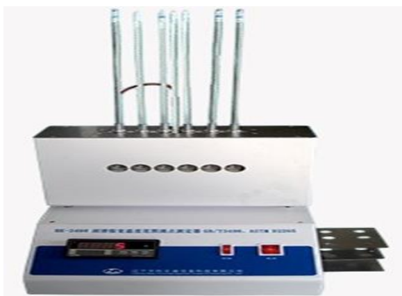
Figure 6 HK-3498 high temperature dropping point equipment (ASTM D2265)
