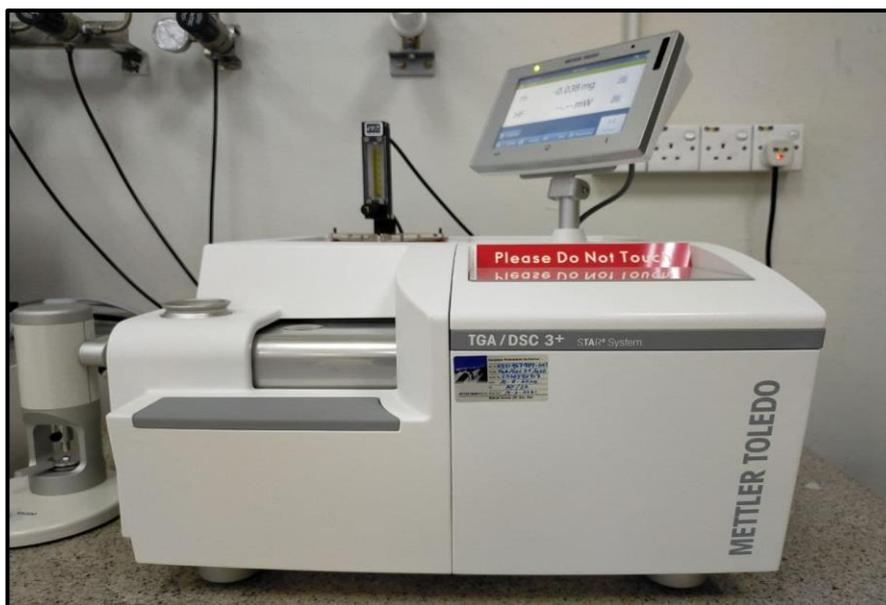
Figure 3.29 TGA device used in the present experimental work
