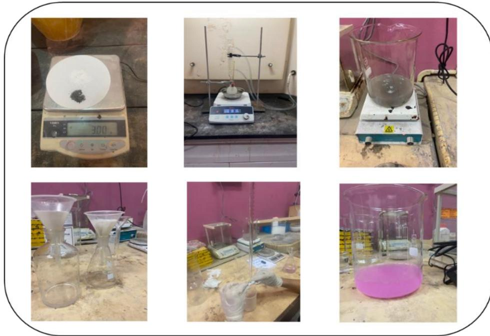
Figure 3.32 Experimental process of the Chapelle test for CBA to check the pozzolanic reactivity
