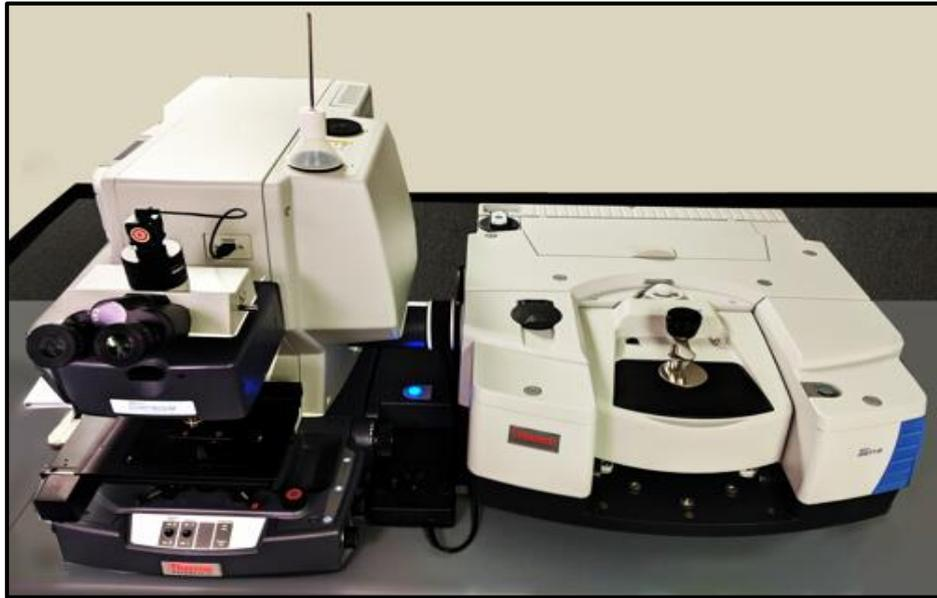
Figure 3.30 FTIR device used in this experimental work
