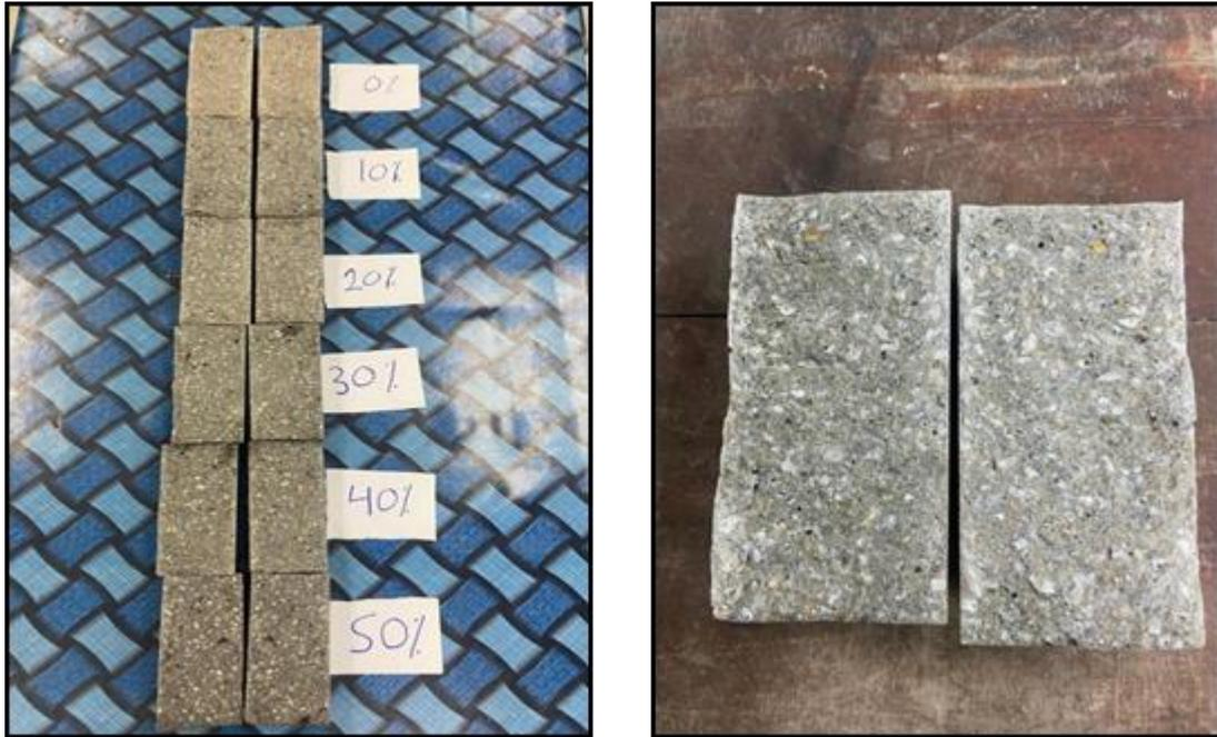
Figure 5.8 Failure occurs through coarse aggregate of SCC mixes containing ground CBA with various replacement ratios
