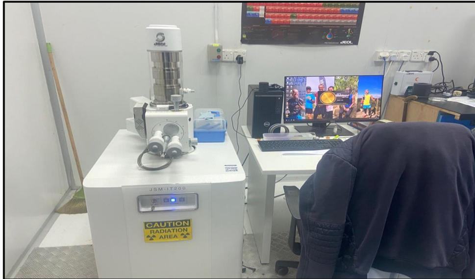
Figure 3.28 SEM used in the present experimental work
