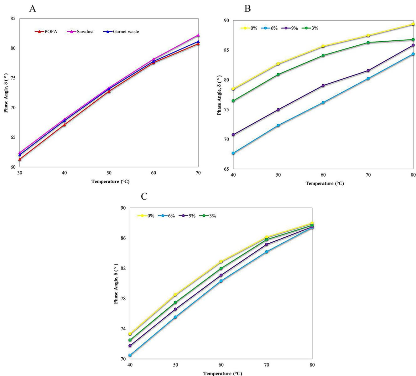
**Fig. 8** a. Phase angle of the 3% POFA-, 3% garnet waste-, and 3% sawdust-modified asphalt binders. b. Phase angle of the 0%, 3%, 6%, and 9% unaged hybrid asphalt binders. c. Phase angle of the 0%, 3%, 6%, and 9% RTFO hybrid asphalt binders
