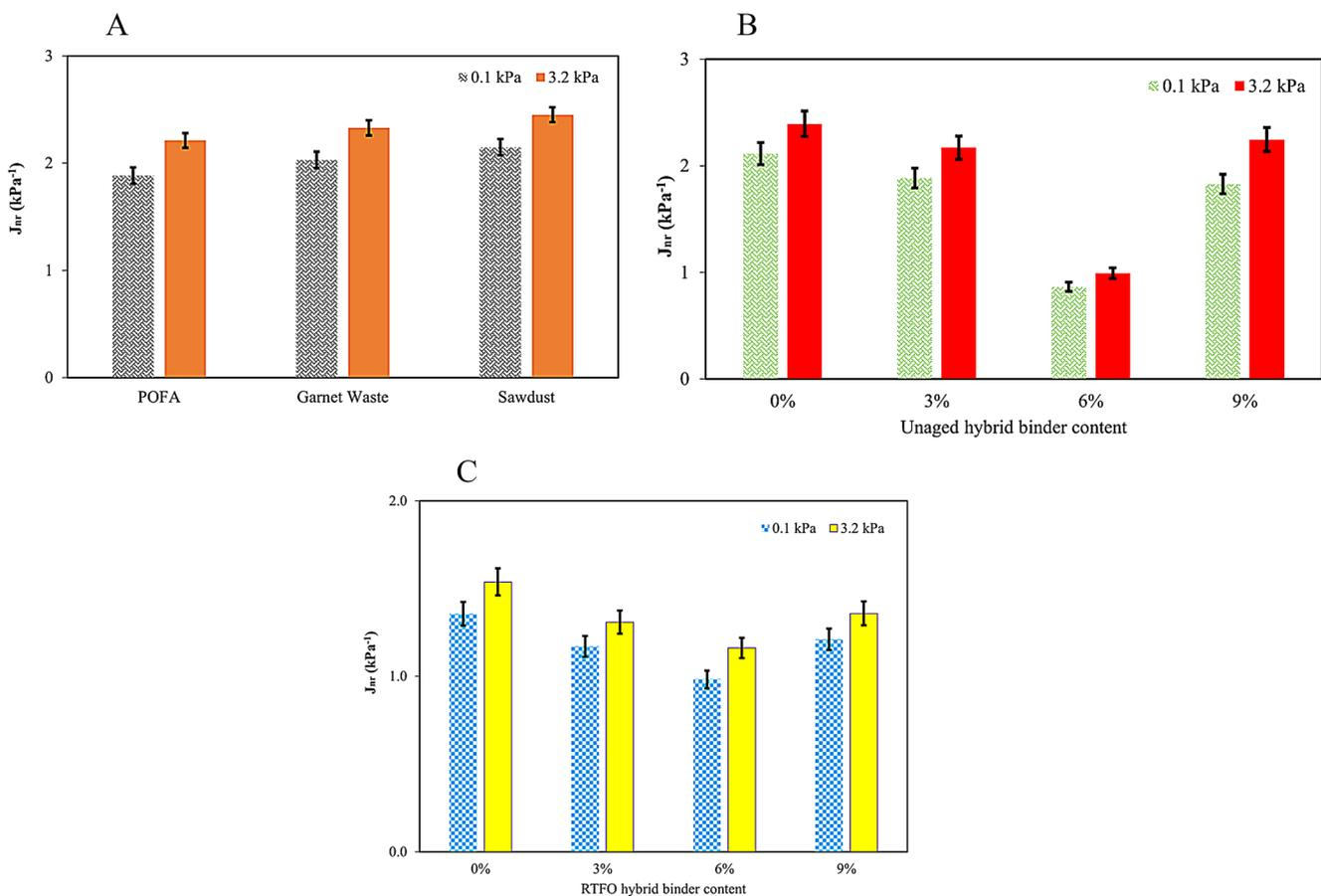
**Fig. 11** a. The  $J_{nr}$  value of the 3% POFA-, 3% garnet waste-, and 3% sawdust-modified asphalt binders at 64°C. b. The  $J_{nr}$  value of the 0%, 3%, 6%, and 9% unaged hybrid asphalt binders at 64°C. c. The  $J_{nr}$  value of the 0%, 3%, 6%, and 9% RTFO hybrid asphalt binders at 64°C
