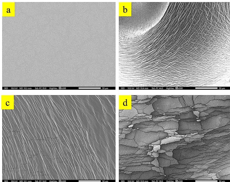
**Fig. 6** The AFM images of hybrid asphalt binder (a) 0%, (b) 3%, (c) 6%, and (d) 9%
