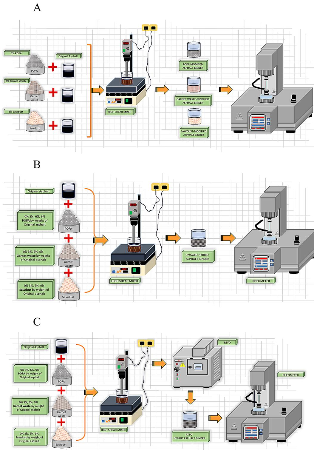
**Fig. 2** a. Blending process of individual-modified asphalt binders for the DSR test. b. Blending process of unaged hybrid asphalt binders for the DSR test. c. Blending process of RTFO hybrid asphalt binders for the DSR test
