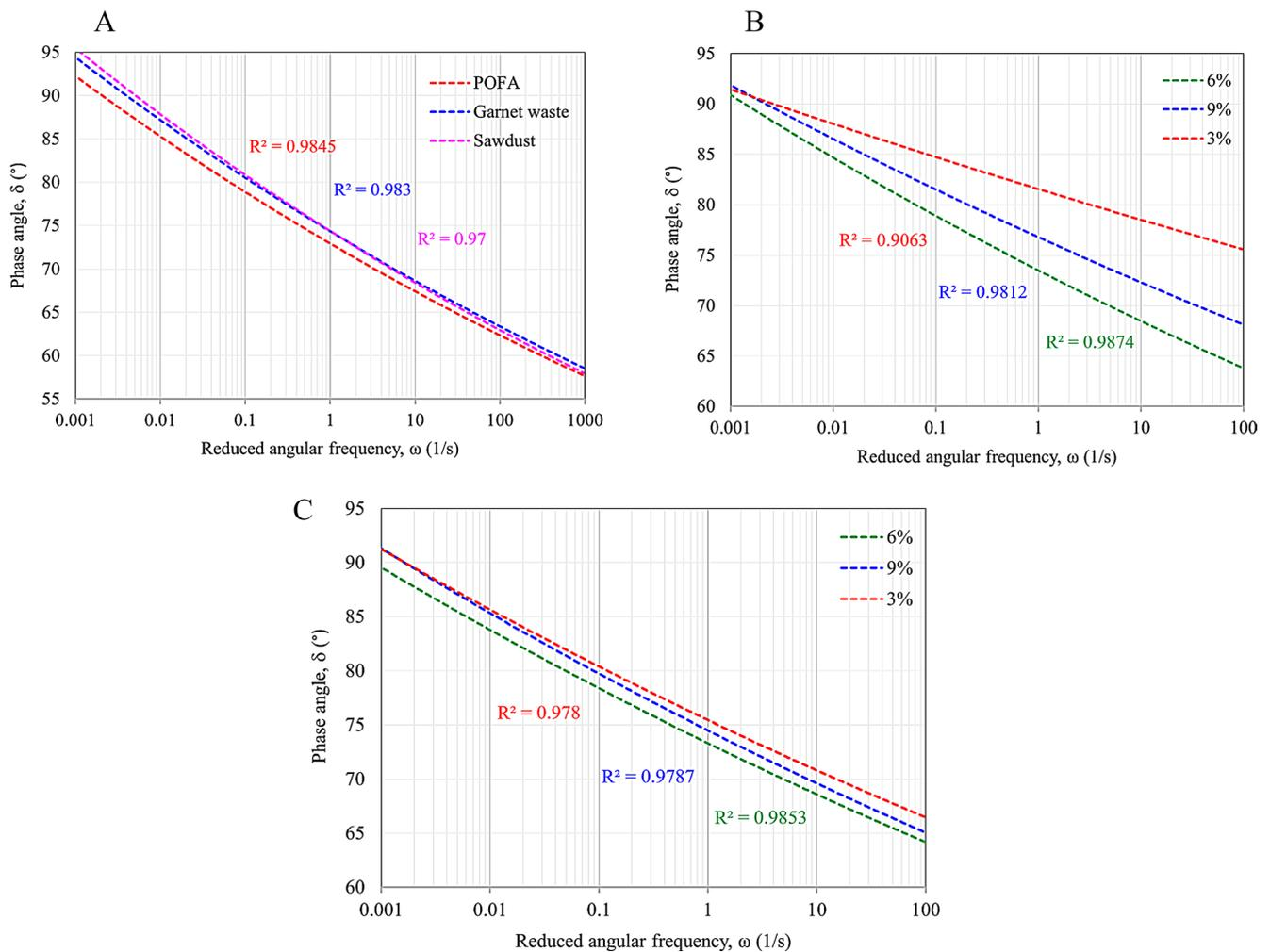
**Fig. 16 a.** Master curve of the phase angle of the 3% POFA-, 3% garnet waste-, and 3% sawdust-modified asphalt binders at 64 °C. **b** Master curve of the phase angle of the 3%, 6%, and 9% unaged hybrid asphalt
