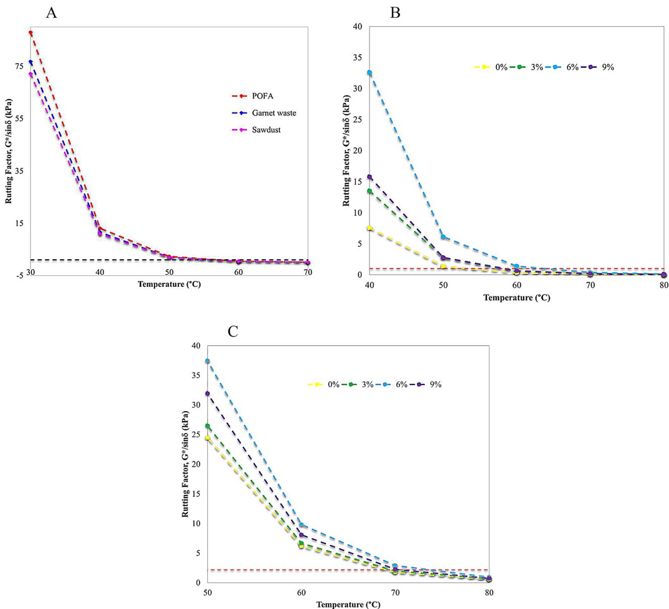
**Fig. 9** a. Rutting factor of the 3% POFA-, 3% garnet waste-, and 3% sawdust-modified asphalt binders. b. Rutting factor of the 0%, 3%, 6%, and 9% unaged hybrid asphalt binders. c. Rutting factor of the 0%, 3%, 6%, and 9% RTFO hybrid asphalt binders
