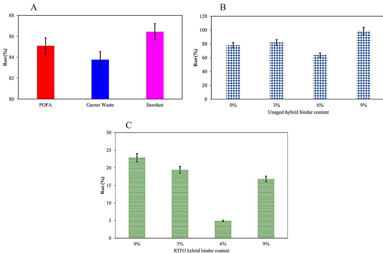
**Fig. 13** a. The  $R_{diff}$  value of the 3% POFA-, 3% garnet waste-, and 3% sawdust-modified asphalt binders at 64 °C. b. The  $R_{diff}$  value of the 0%, 3%, 6%, and 9% unaged hybrid asphalt binders at 64 °C. c. The  $R_{diff}$  value of the 0%, 3%, 6%, and 9% RTFO hybrid asphalt binders at 64 °C
