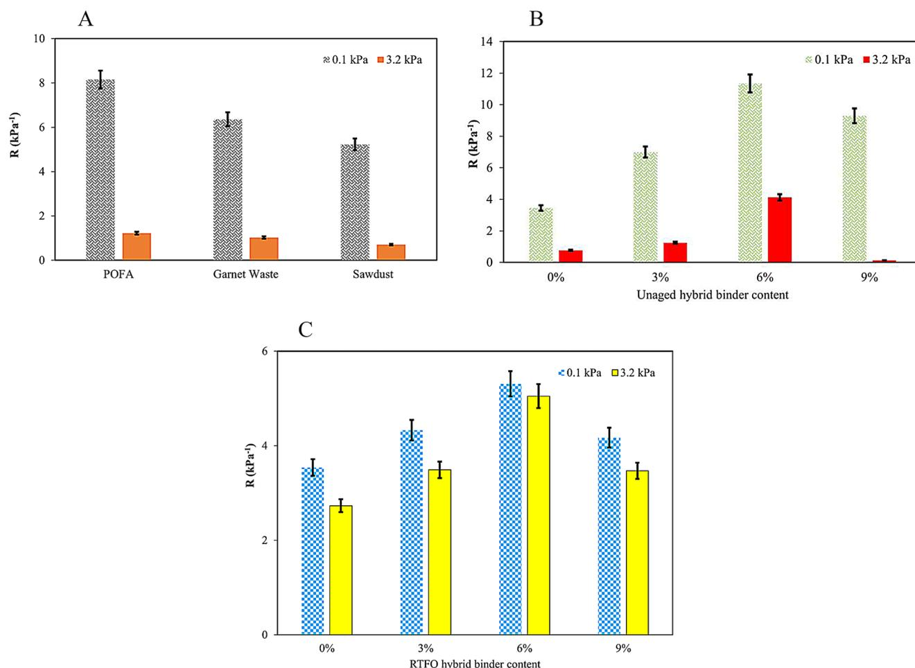
**Fig. 12** a. The R-value of the 3% POFA-, 3% garnet waste-, and 3% sawdust-modified asphalt binders at 64 °C. b. The R-value of the 0%, 3%, 6%, and 9% unaged hybrid asphalt binders at 64 °C. c. The R-value of the 0%, 3%, 6%, and 9% RTFO hybrid asphalt binders at 64 °C
