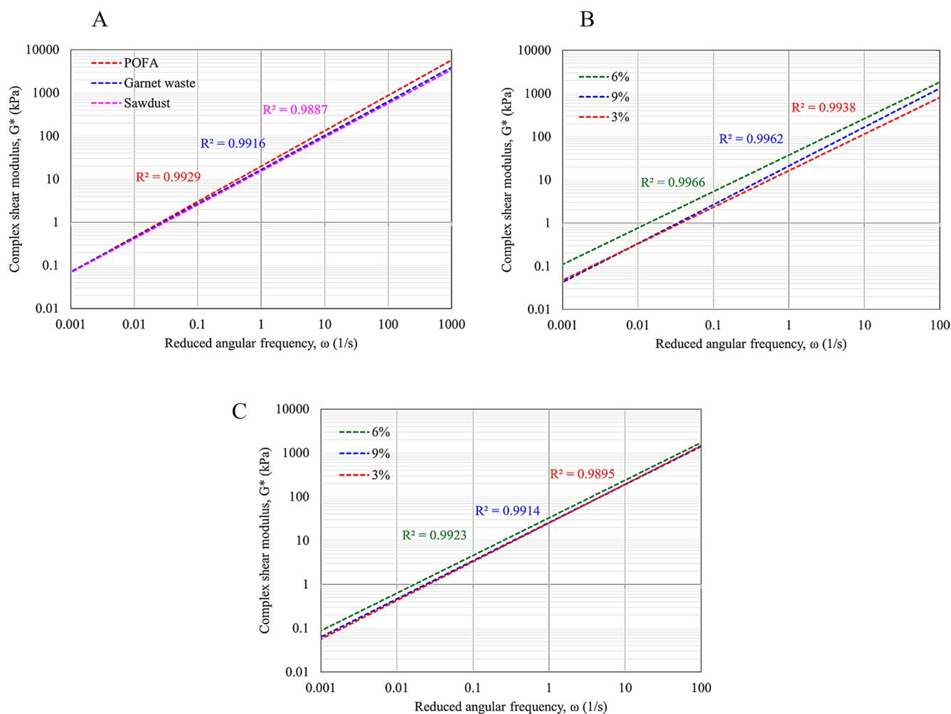
**Fig. 15 a.** Master curve of the complex shear modulus of the 3% POFA-, 3% garnet waste-, and 3% sawdust-modified asphalt binders at 64 °C. **b** Master curve of the complex shear modulus of the 3%, 6%,
