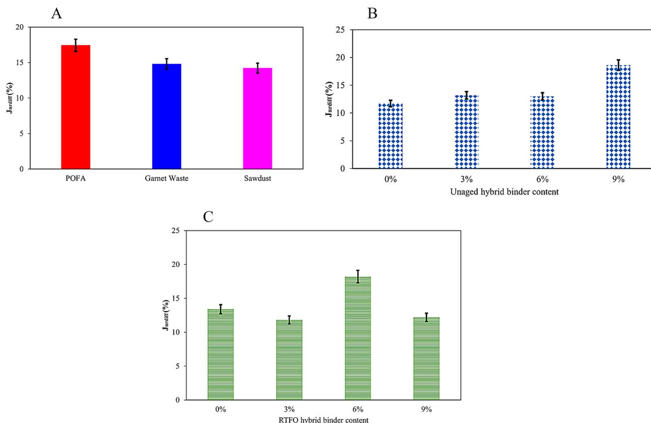
**Fig. 14** a. The  $J_{nr,diff}$  value of the 3% POFA-, 3% garnet waste-, and 3% sawdust-modified asphalt binders at 64 °C b. The  $J_{nr,diff}$  value of the 0%, 3%, 6%, and 9% unaged hybrid asphalt binders at 64 °C. c. The  $J_{nr,diff}$  value of the 0%, 3%, 6%, and 9% RTFO hybrid asphalt binders at 64 °C
