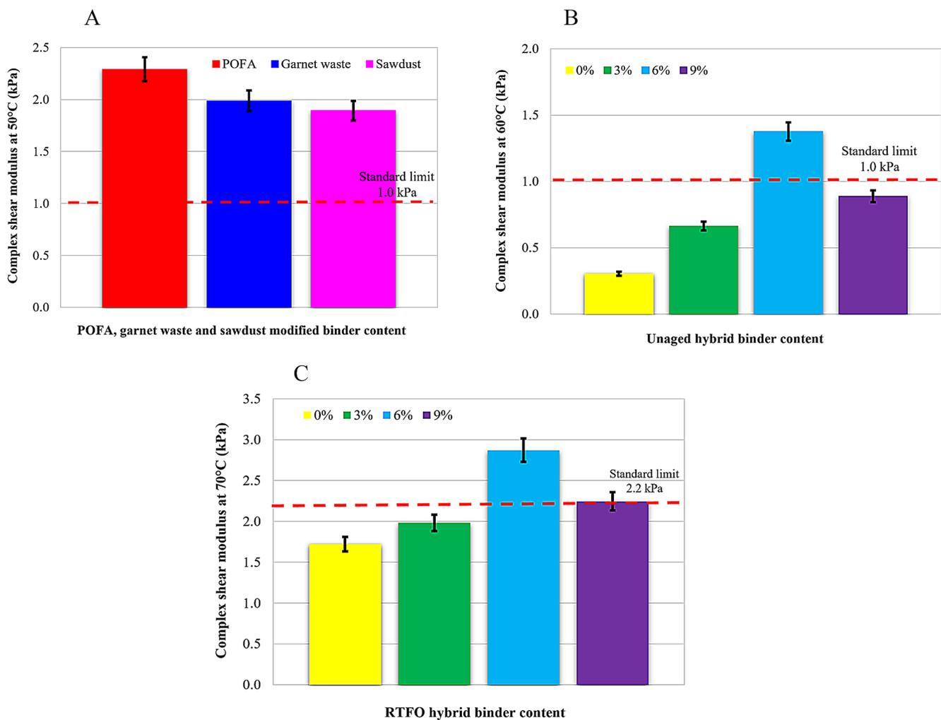
**Fig. 7** a. Complex shear modulus of the 3% POFA-, 3% garnet waste-, and 3% sawdust-modified asphalt binders. b. Complex shear modulus of the 0%, 3%, 6%, and 9% unaged hybrid asphalt binders. c. Complex shear modulus of the 0%, 3%, 6%, and 9% RTFO hybrid asphalt binders
