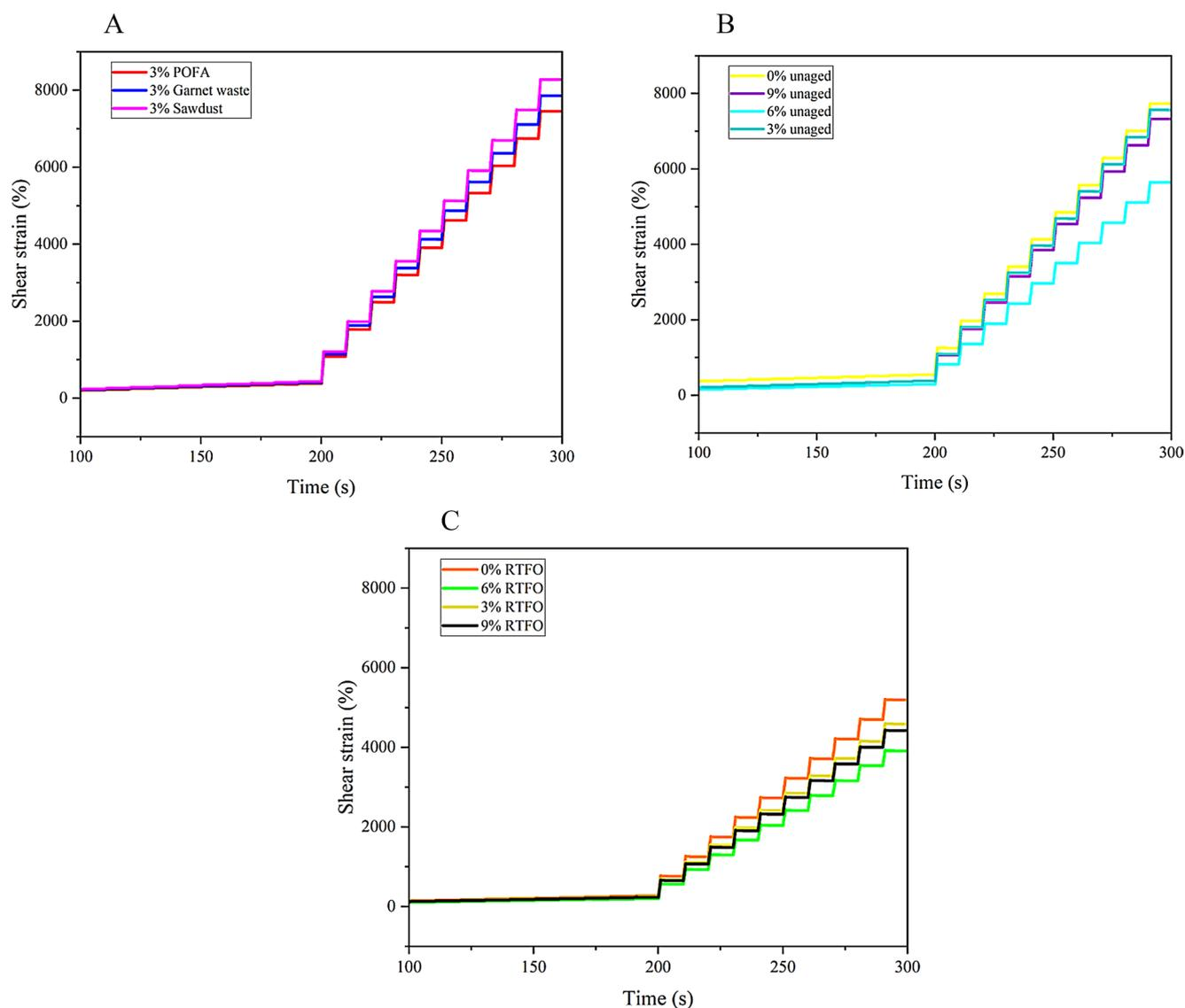
**Fig. 10** a. MSC R strain curve of the 3% POFA-, 3% garnet waste-, and 3% sawdust-modified asphalt binders. b. MSCR strain curve of the 0%, 3%, 6%, and 9% unaged hybrid asphalt binders. c. MSCR strain curve of the 0%, 3%, 6%, and 9% RTFO hybrid asphalt binders
