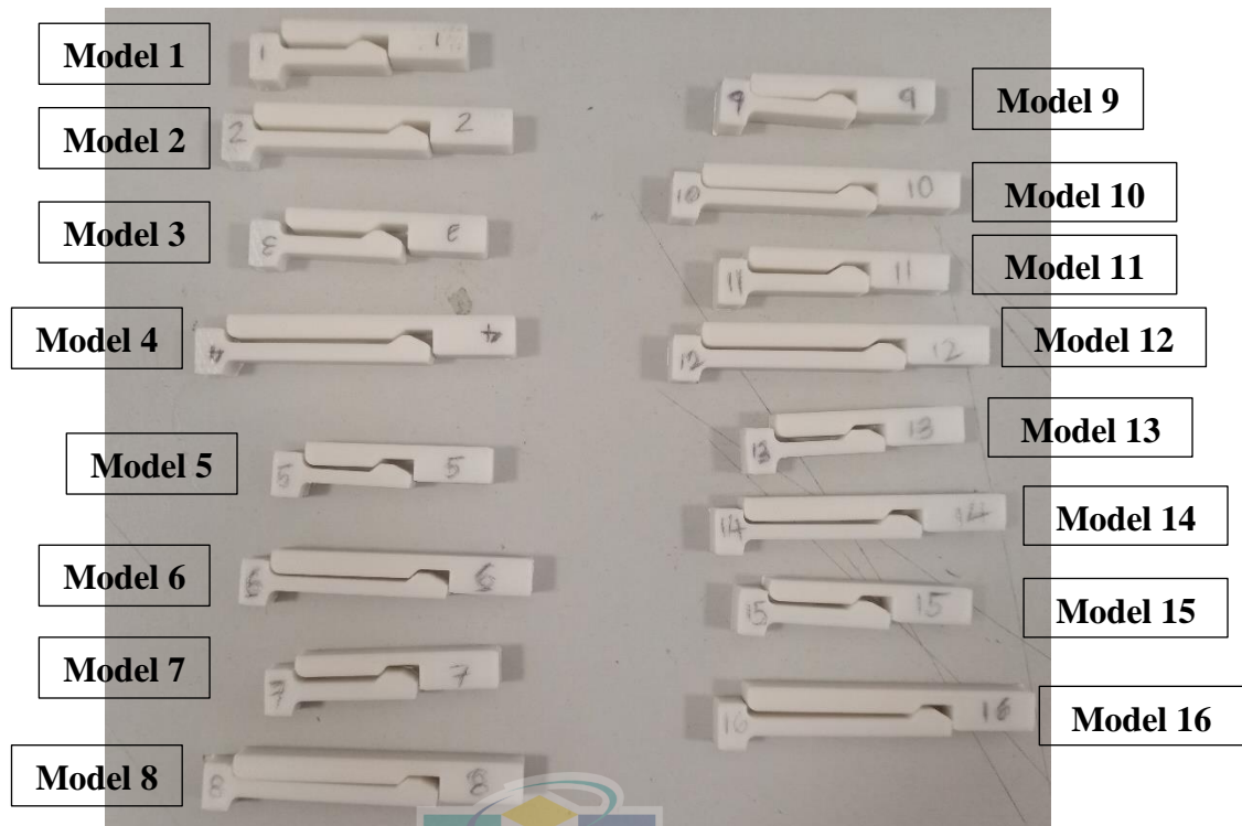
Figure 3.18 16 Models of Snap-fits
