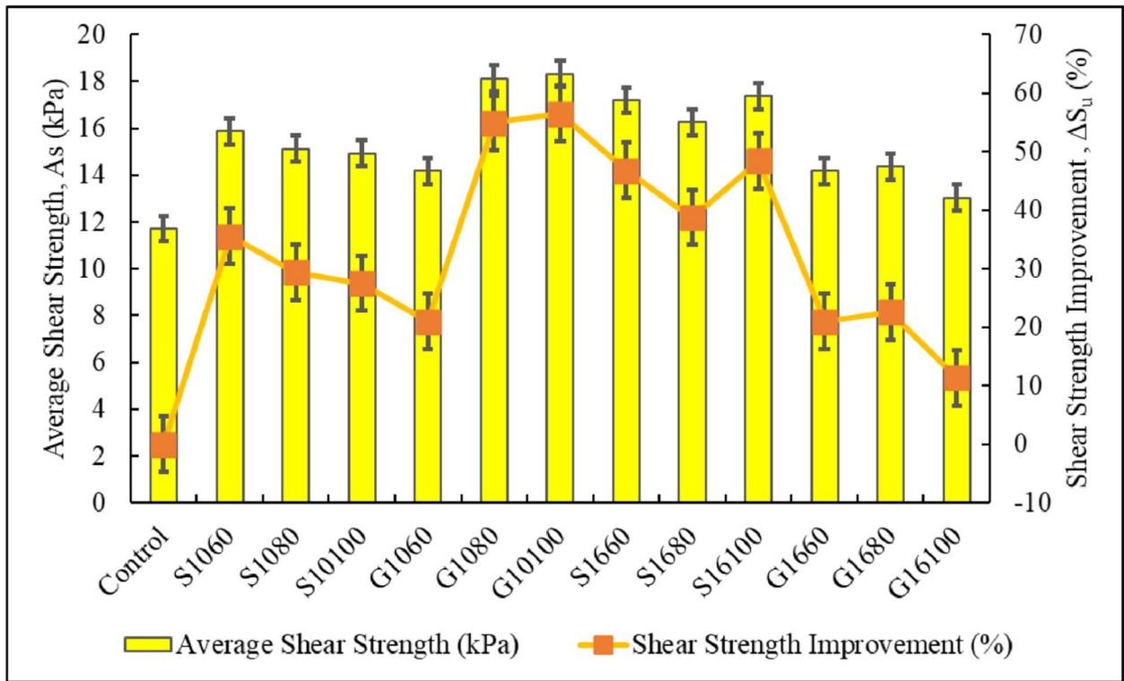
**Fig. 8** Results of the UCT. (a) Shear strength improvement of kaolin clay after the installation of single or group PET columns. Green values = the highest recorded improvement values; red values = the low-
