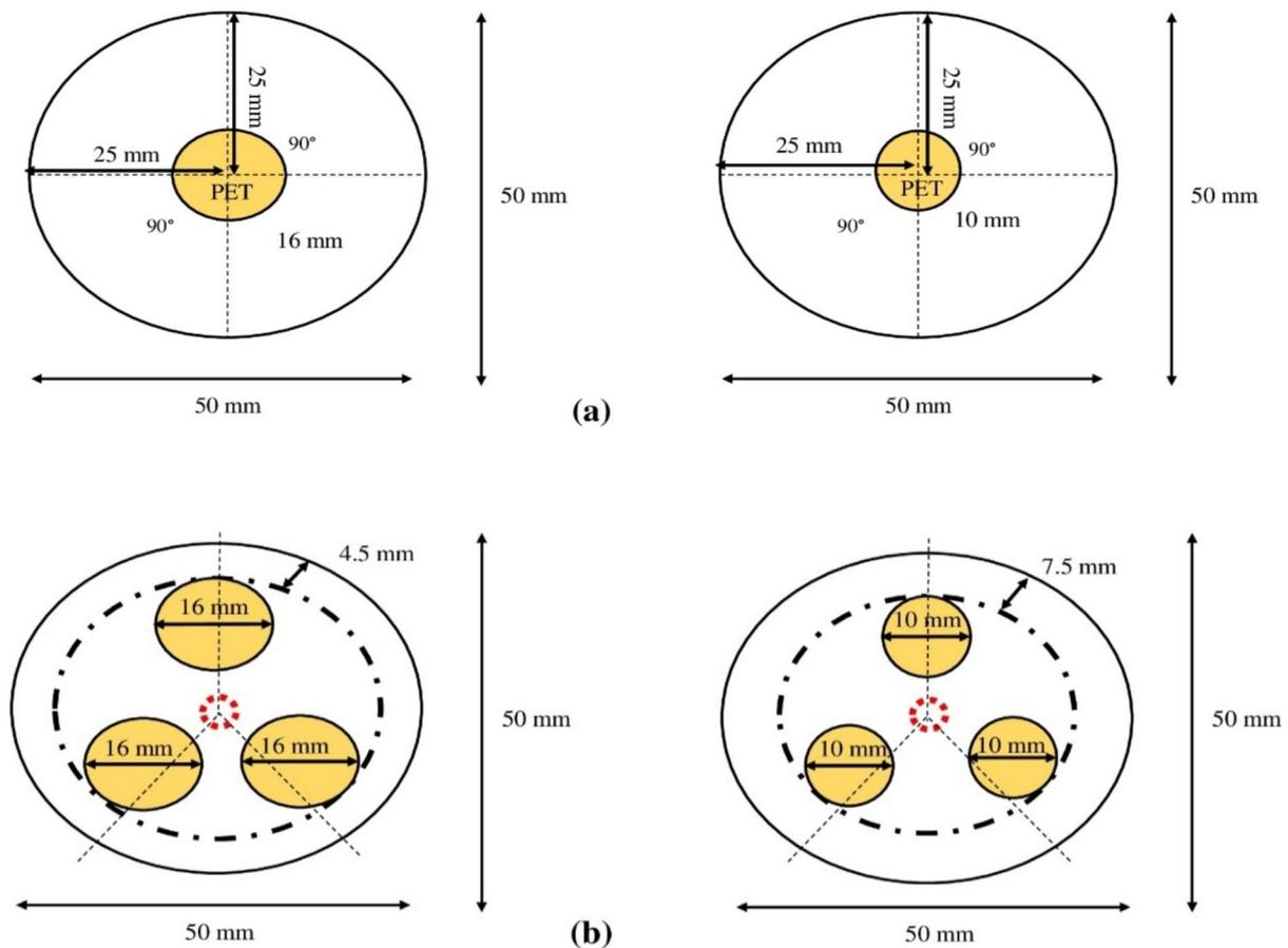
Fig. 3 Detailed arrangement of (a) the single PET column and (b) the group PET columns
