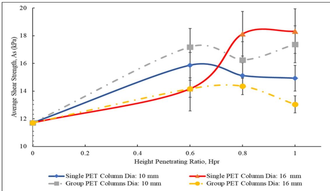
**Fig. 10** The relationship between the average shear strength value ( $A_s$ ) and the height penetrating ratio ( $H_{pr}$ ) for the single and group PET columns
