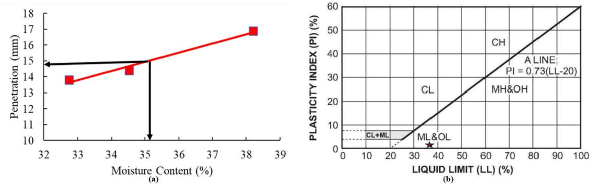
**Fig. 6** Atterberg limit: (a) 20 mm cone penetration, (b) USCS chart for soil classification
