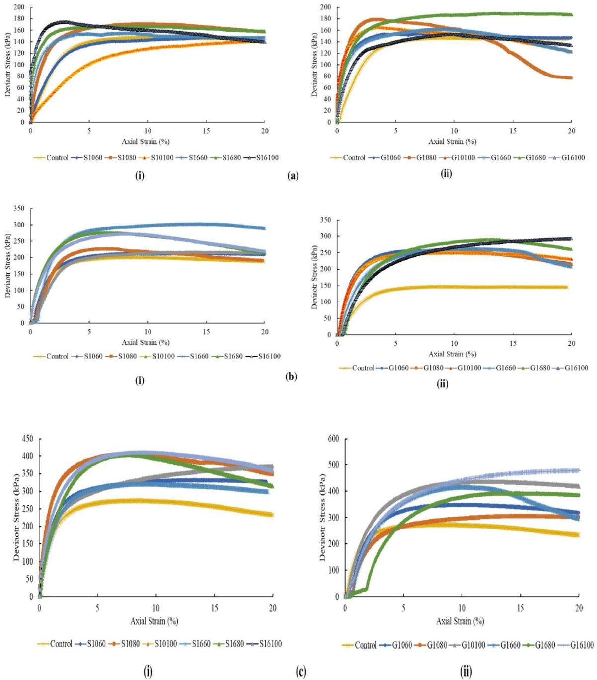
**Fig. 13** The results obtained from the unconsolidated undrained test for the single and group PET columns at confining pressure of (a) 100 kPa, (b) 200 kPa, and (c) 400 kPa. (i) Single PET column. (ii) Group PET column. S, single; G, group
