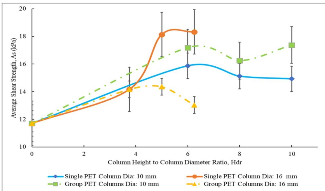
**Fig. 11** The relationship between the average shear strength value ( $A_s$ ) and the column height-to-column diameter ratio ( $H_{dr}$ ) for the single and group PET columns
