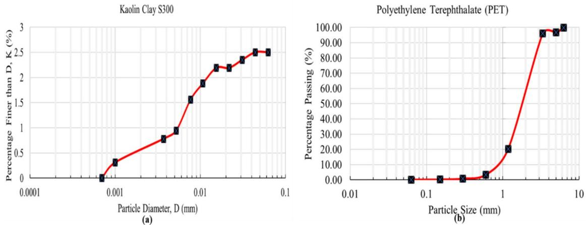
**Fig. 5** The particle size distribution of (a) kaolin clay S300 and (b) PET plastic
