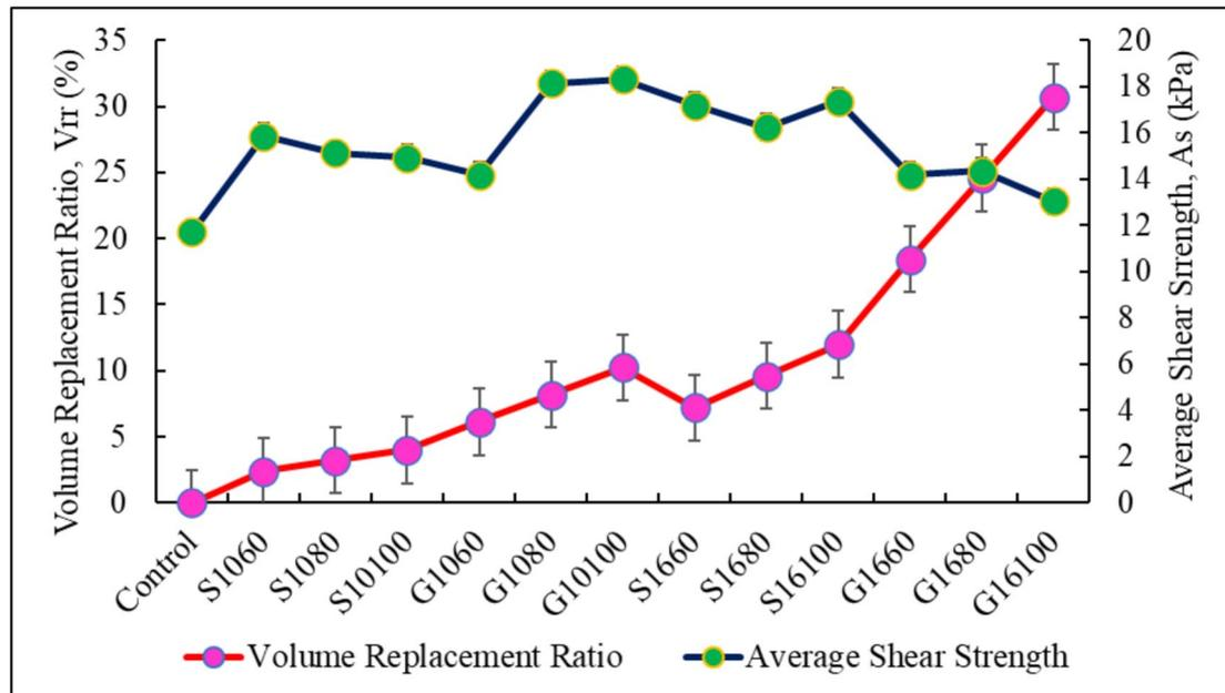
**Fig. 12** The relationship between the average shear strength value ( $A_s$ ) and the volume replacement ratio ( $V_{rr}$ ) for the single and group PET columns
