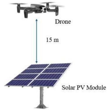
FIGURE 6. Acquisition of height for the image capture procedure.
