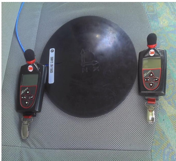
Figure 3.7: Accelerometer sensor and dosimeter used for measuring the vibration.
