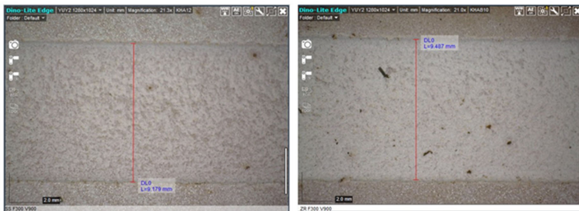
Fig. 6. Maximum groove lengths after machining the cuts from f = 0.03 mm/tooth and s = 900 m/min SS316 (left) and ZrO_2 (right)
