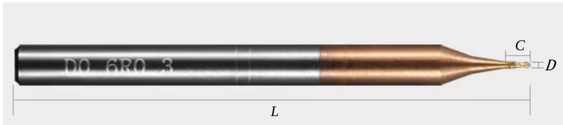
Figure 3.11 Micromilling tool geometry
