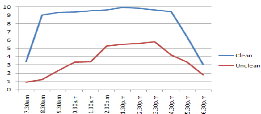
Figure 4.11: Cleaned single axis tracker versus unclean single axis tracker graph.
