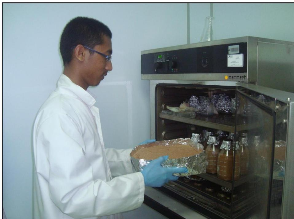
**Figure 3.4:** Drying the sawdust
