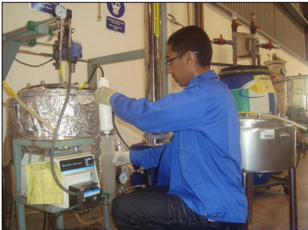
**Figure 3.12:** Separation of glucose using ultrafiltration membrane
