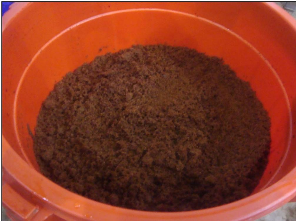
**Figure 3.7:** Sawdust after Sodium Hydroxide pretreatment
