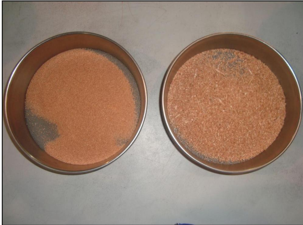
**Figure 3.3:** Sawdust before and after sieving
