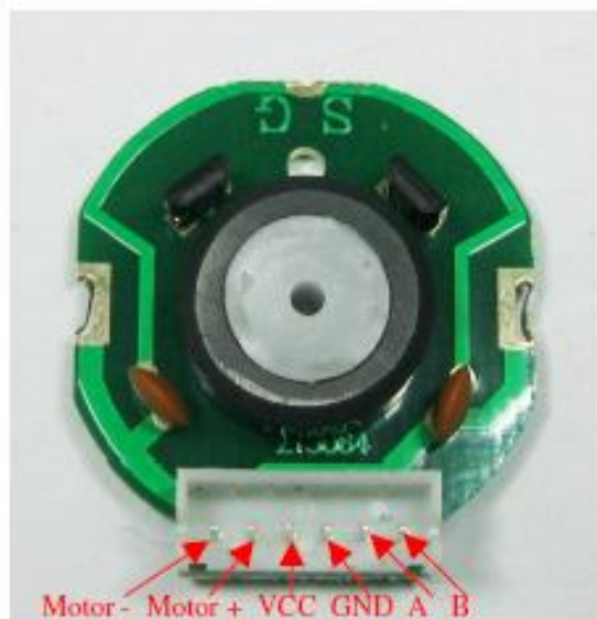
Figure 2.0 2020-06 connector pin descriptions
