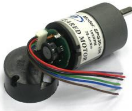
Figure 1.0 DC geared motor with encoder and its removable cover
