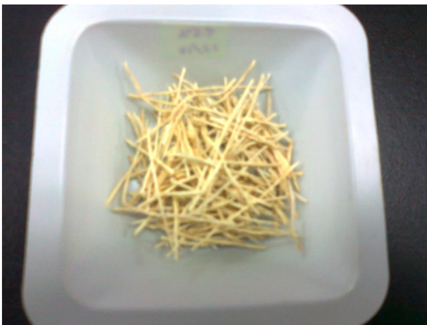
Figure 3.3: Squeezed and Dried Oil Palm Trunk (OPT) Fiber
