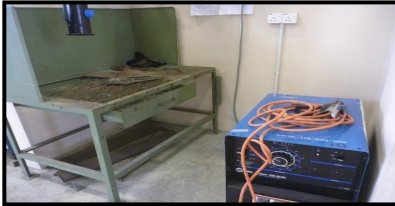
Figure 3.8: Shield Metal Arc Weld (SMAW)
