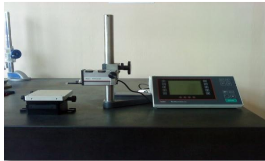
Figure 3.4: Mahr Perthometer S2 used in the present study
