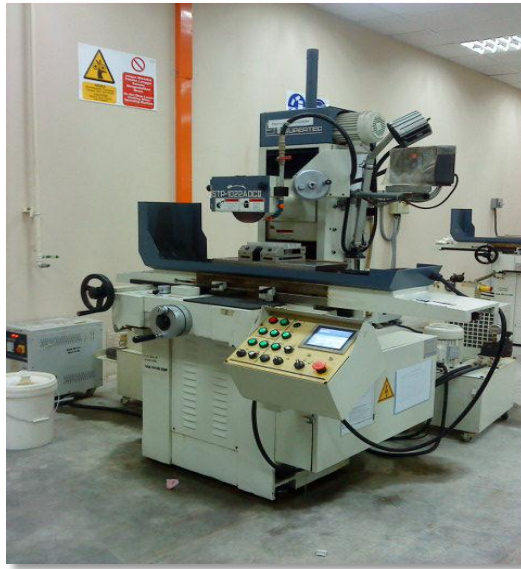
Figure 3.2: Surface grinding machine used in the present study.
