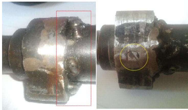
Figure 4.8: Welding and Pin at Camshaft.
