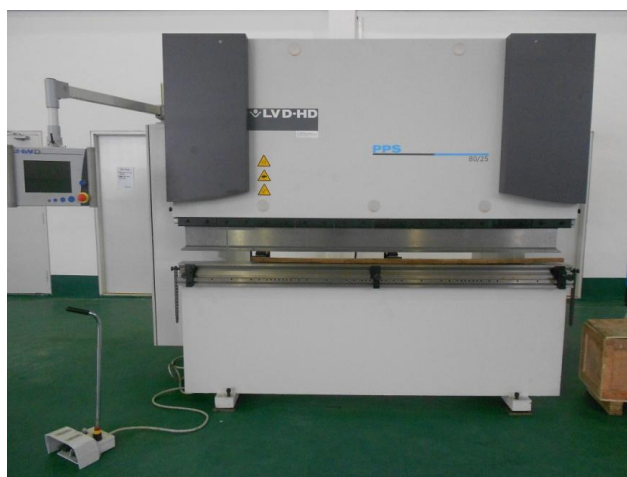
Figure 3.11: LVD-HD bending machine
