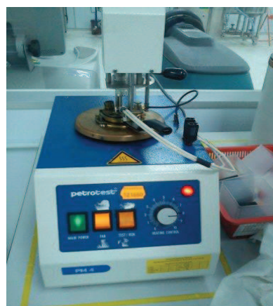
Figure 3.10: Petrotest Flash Point & Auto ignition tester
