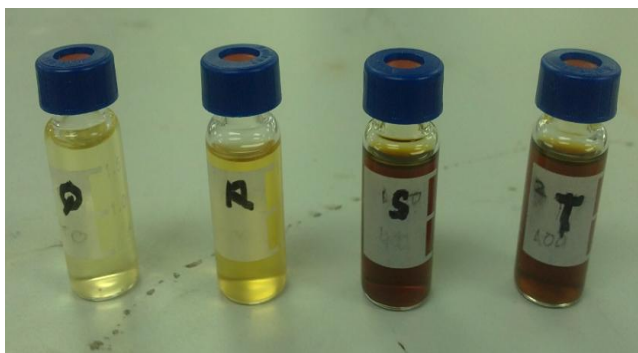
Figure 4.9 : Sample 3 (Cracking at 400°C)
