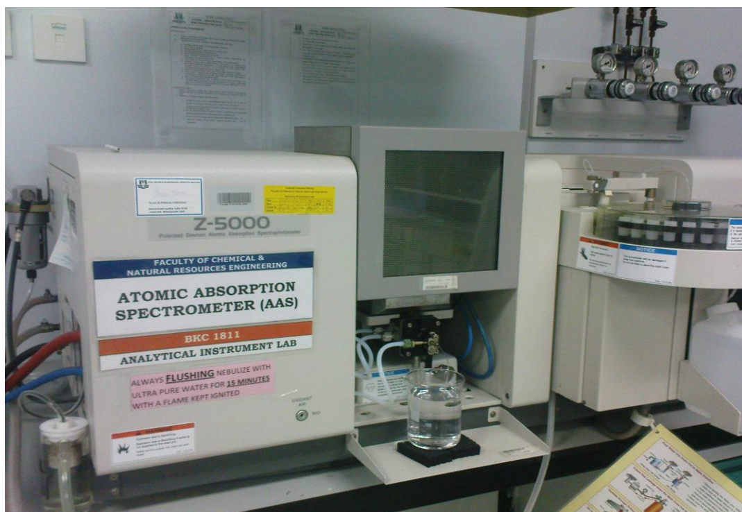
Figure 5 Atomic Absorption Spectrometer (AAS) for analysis
