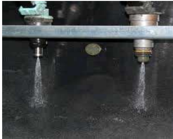
Figure 6.2: Test the injector maximum pressure
