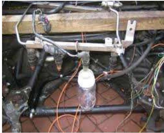
Figure 6.1: Set-up the common rail
