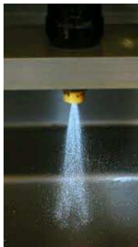
Figure 6.5: Test high pressure of the injector
