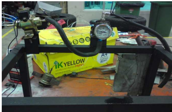
Figure 6.7: Set the fuel pump pressure with fuel regulator
