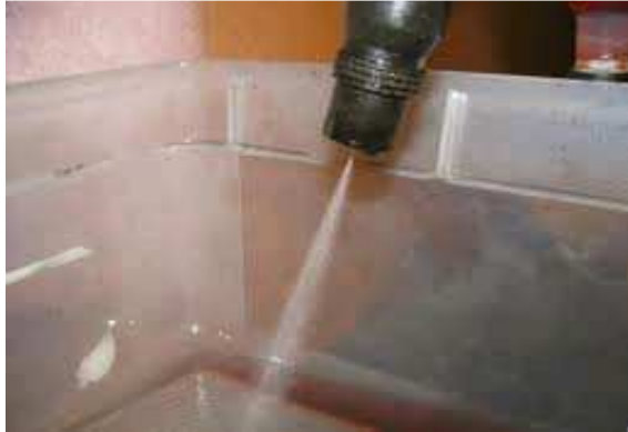
Figure 6.3: Test the injector pressure
