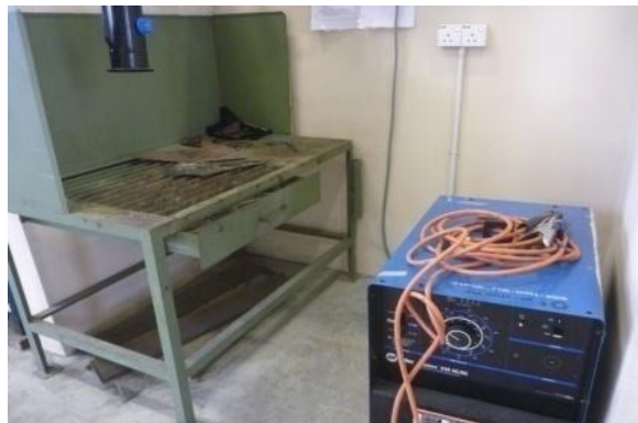
Figure 3.5: SMAW weld Equipment
