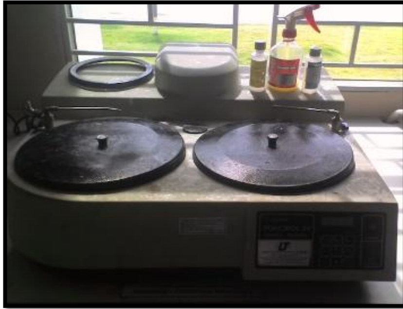
Figure 3.4: (ii) Sample preparations polishing with 6 \mu Polycrystalline diamond polishing with 3 \mu Polycrystalline diamond and 1 \mu Polycrystalline diamond.
