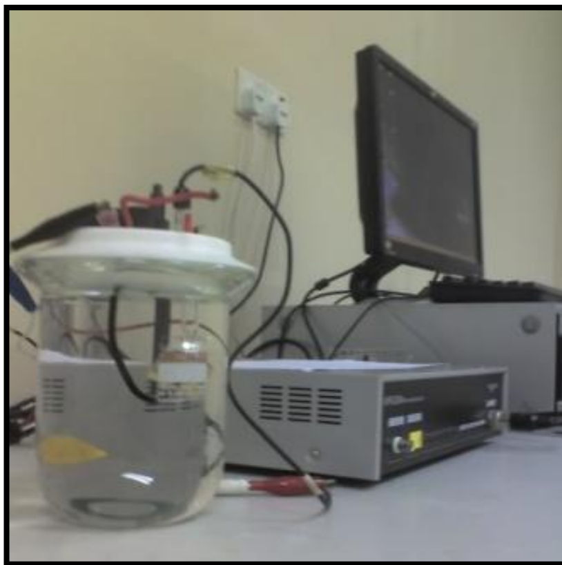
Figure 3.7: Electrochemical cells interconnect with WPG 100 potentiostat and computer.
