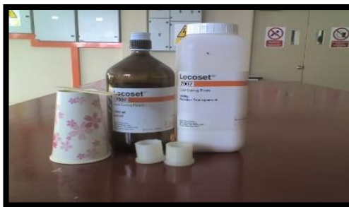
(a) cold mounting and embed the Copper wire
