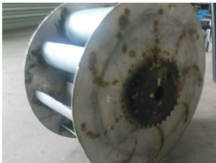
Figure 3.11: Complete assemble of the stainless steel propeller model
