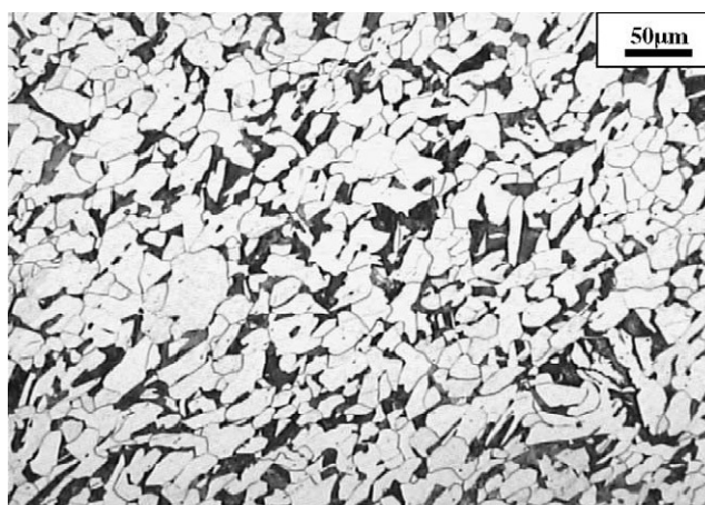
Figure 2.3 : Microstructure as-receive of AISI 1020
