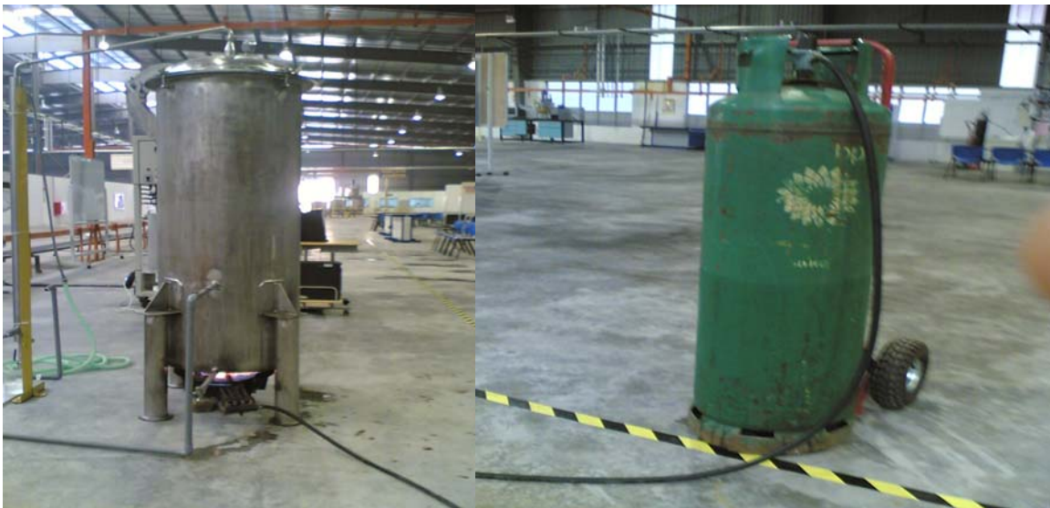
Figure 3.2: The Steam Distillation Equipment
