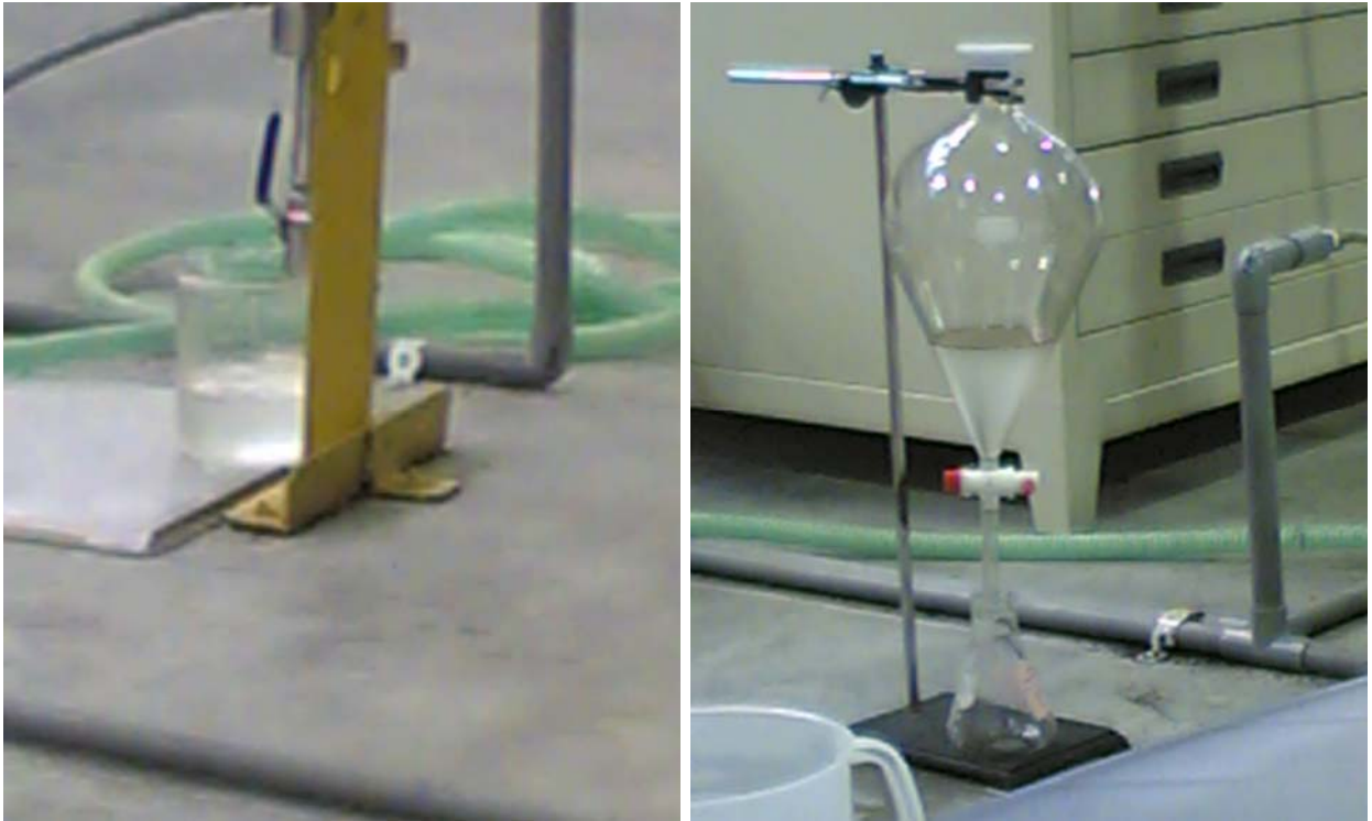
Figure 3.3: The Ginger Essential Oil Is Collected and Separated
