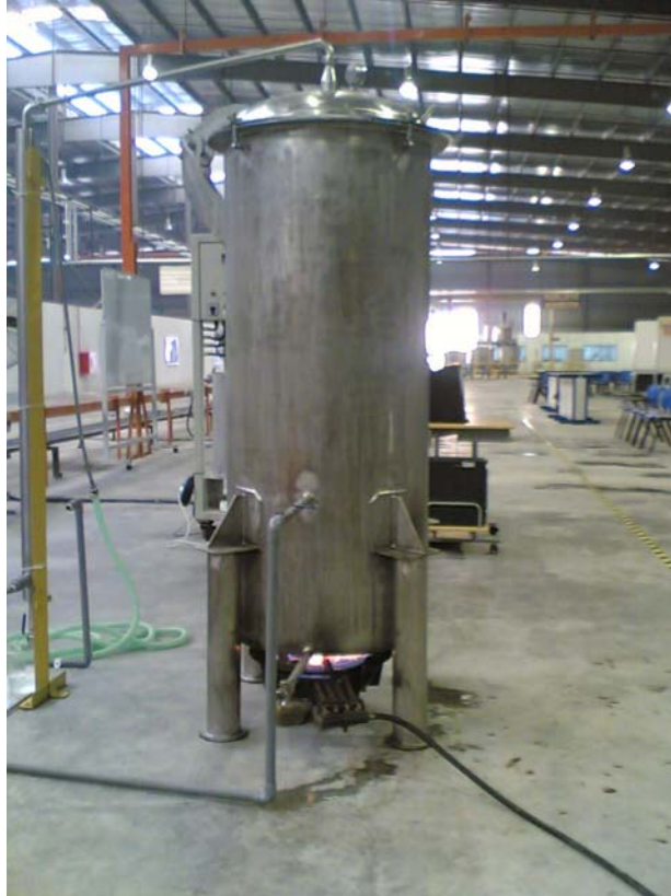
Figure 2.8: Steam Distillation Pilot Plant
