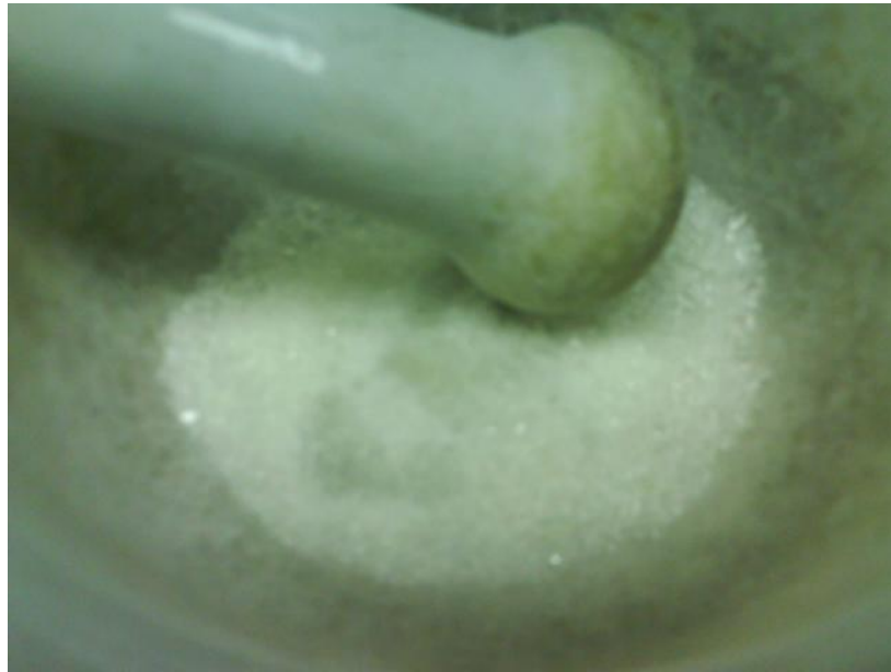
Figure D.1 Ground polymer with mortar and pestle.
