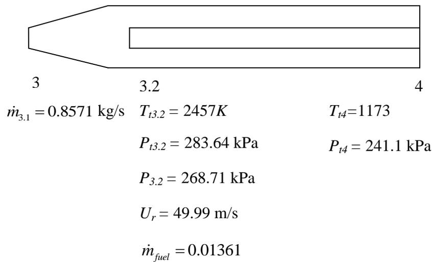
**Figure 3.4:** Summary of calculated and assumed parameter at different station in the combustion chamber
