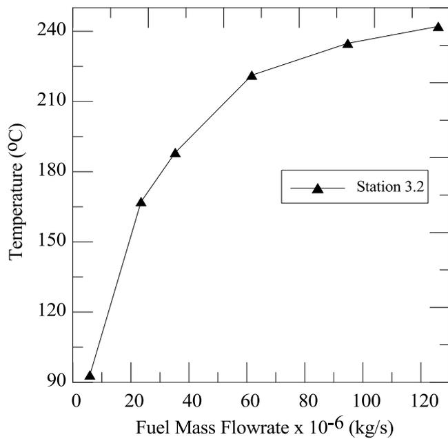
**Figure 4.9:** Graph of temperature mass flow rate at station 3.2
