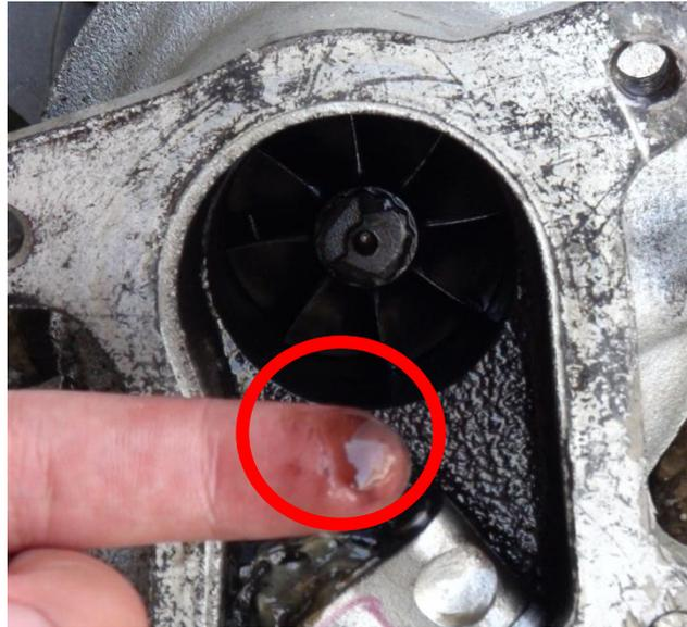
**Figure 4.13:** Lubricant oil leaks at the turbine blades
