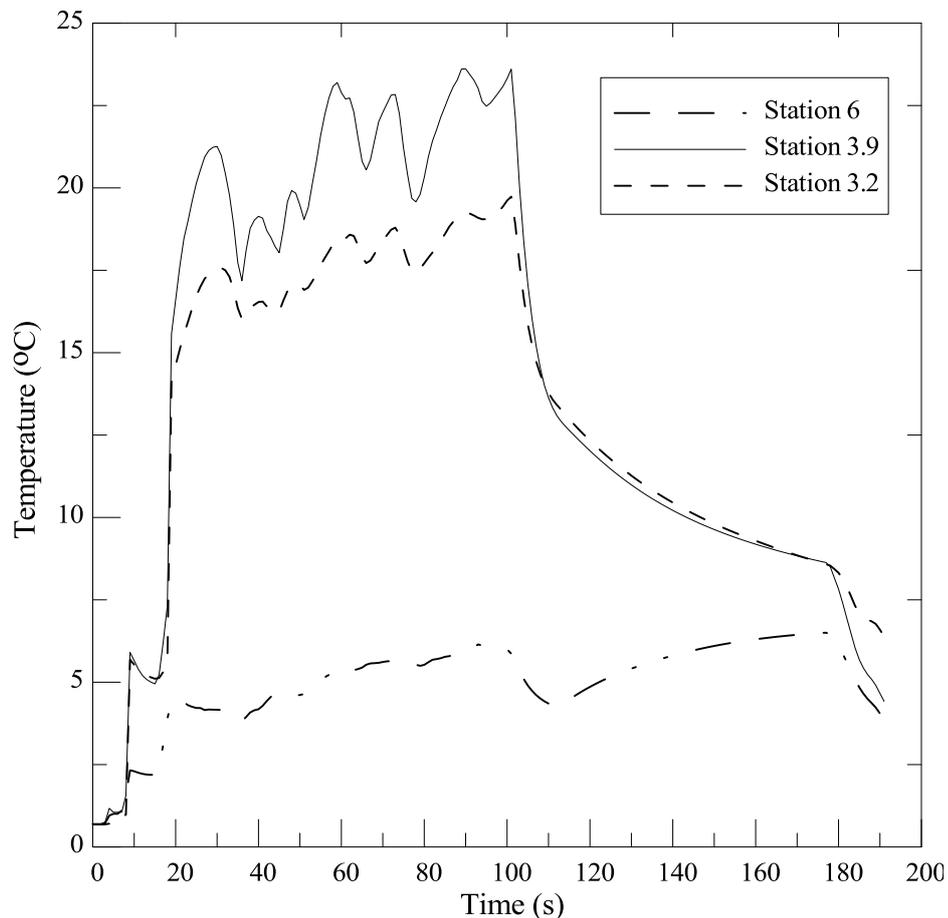
**Figure 4.8:** Graph of temperature distribution of the jet engine at 3 different stations during testing period
