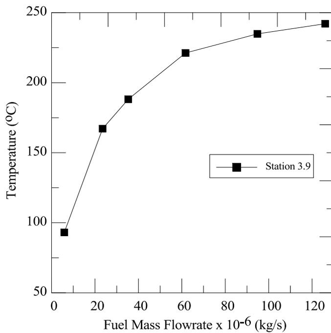
**Figure 4.10:** Graph of temperature mass flow rate at station 3.9
