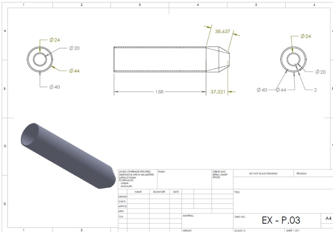
**Figure 6.8:** Two-dimensional drawings of assembled exhaust nozzle
