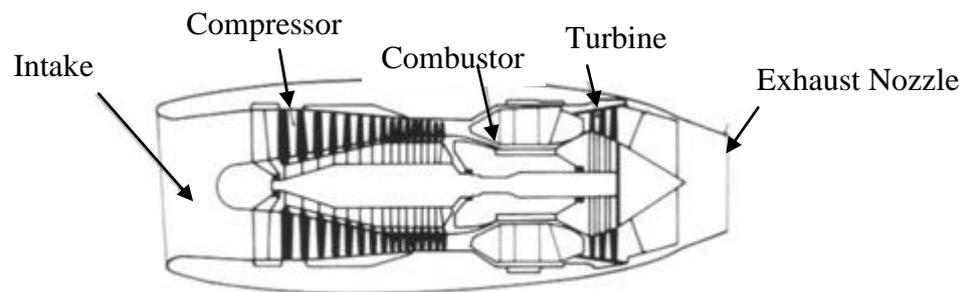
**Figure 2.2:** Schematic illustration of turbojet engine
