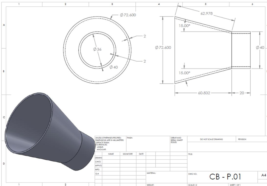
**Figure 6.1:** Two-dimensional drawing of inlet diffuser
