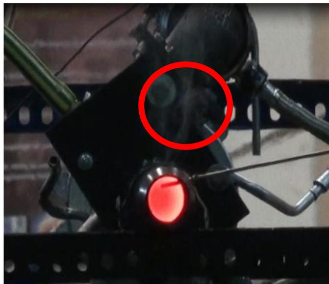
**Figure 4.14:** White smoke appear at the turbine housing during testing
