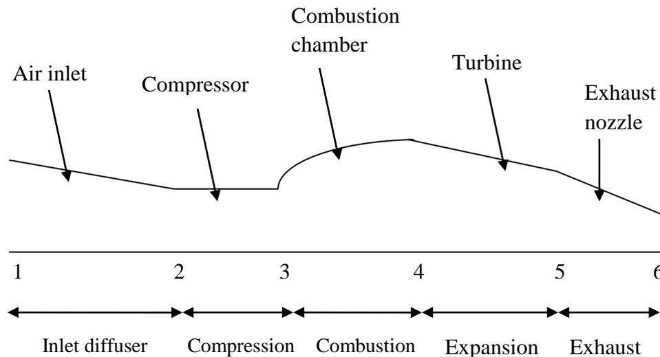
**Figure 2.5:** Schematic diagram of jet-propulsion cycle. The number represents the engine station locations and will be used throughout this report
