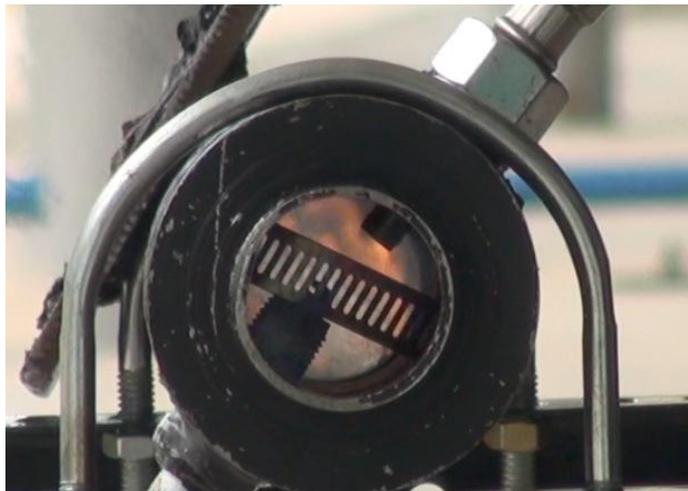
**Figure 4.6:** Flame contained inside the combustion chamber
