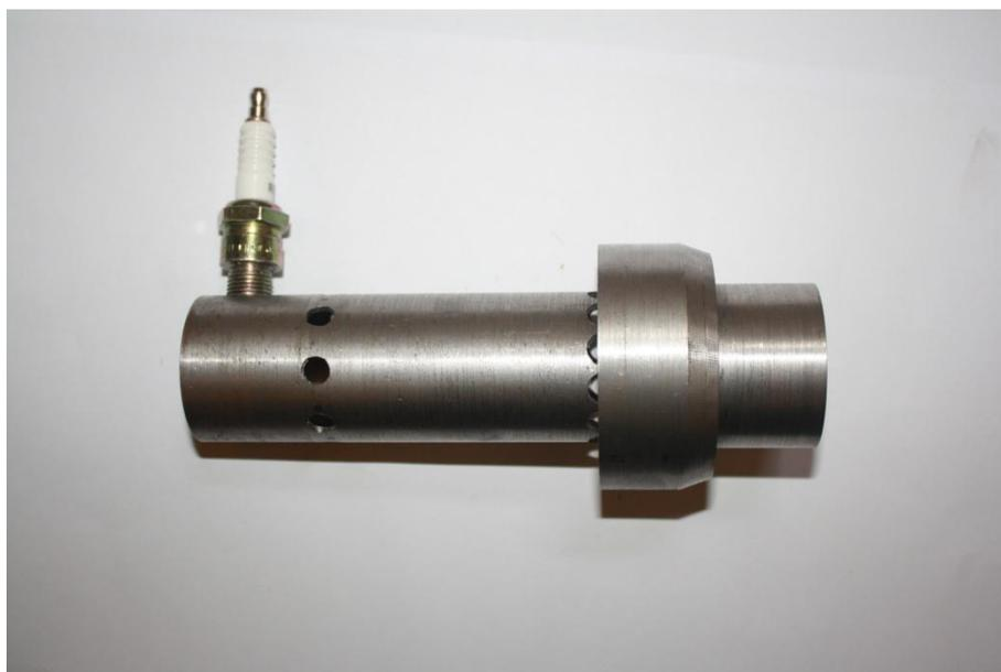
**Figure 3.12:** Fabricated inner liner with spark plug and holder attached
