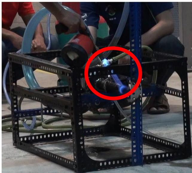
**Figure 4.3:** Method of ignition by lighter at the exhaust
