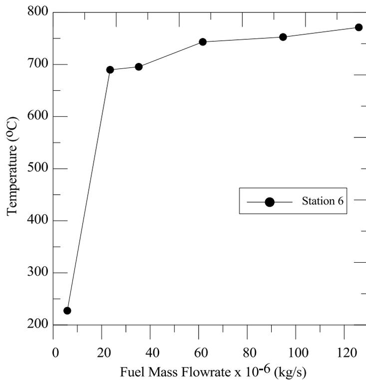
**Figure 4.11:** Graph of temperature versus fuel mass flow rate at station 6
