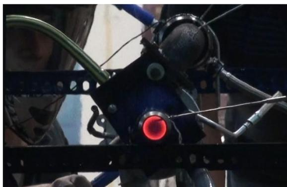
**Figure 4.7:** Turbine blade glowing red
