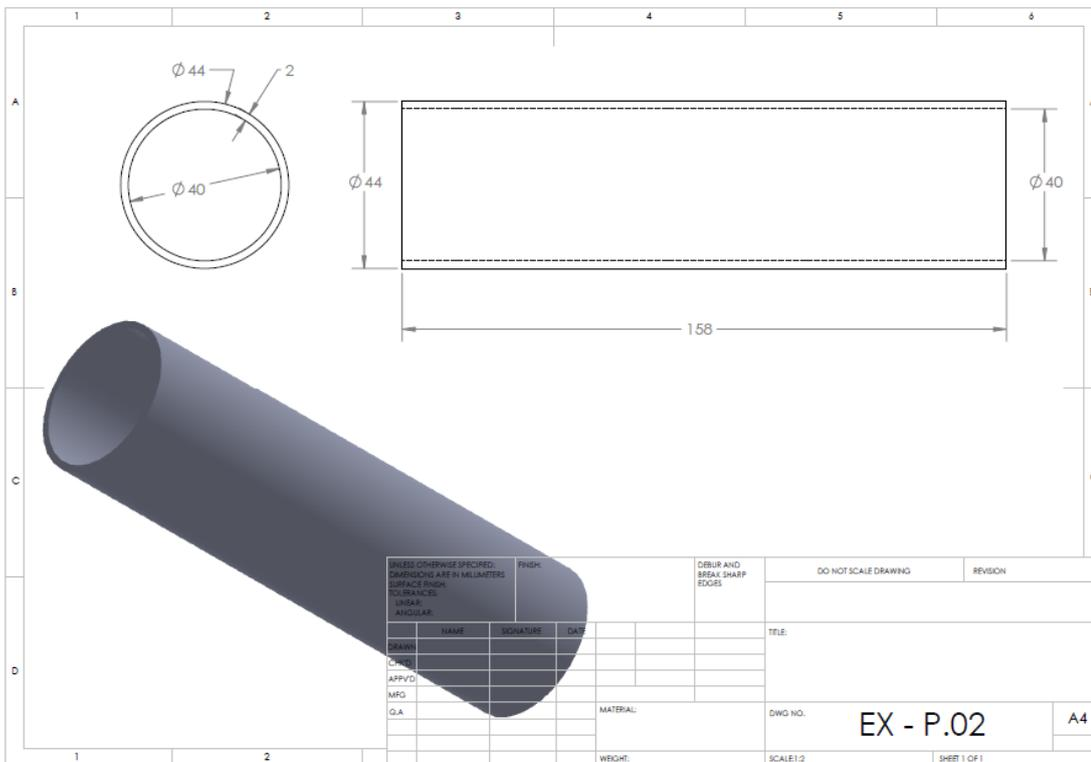
**Figure 6.7:** Two-dimensional drawings of exhaust liner
