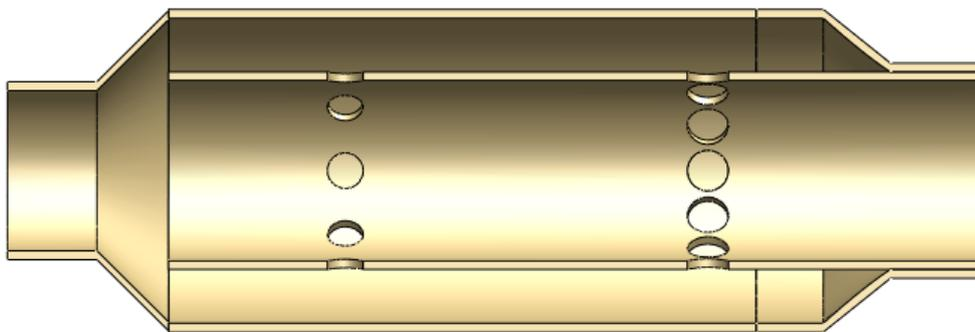
**Figure 3.7:** Sectional view of combustion chamber
