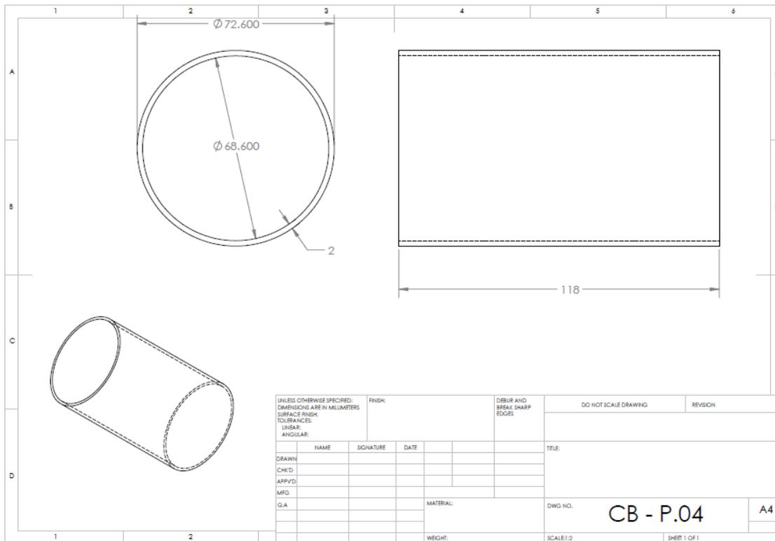
**Figure 6.4:** Two-dimensional drawing of outer liner
