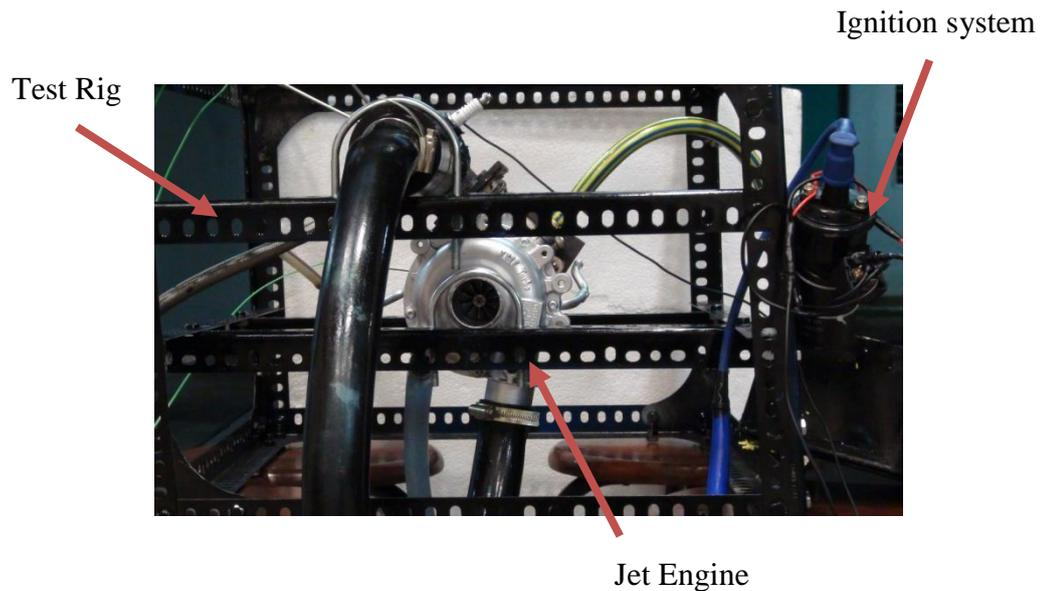
**Figure 3.17:** Jet engine mounted on a test rig
