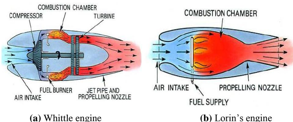
**Figure 2.1:** Comparison between Lorin's and Whittle engine
