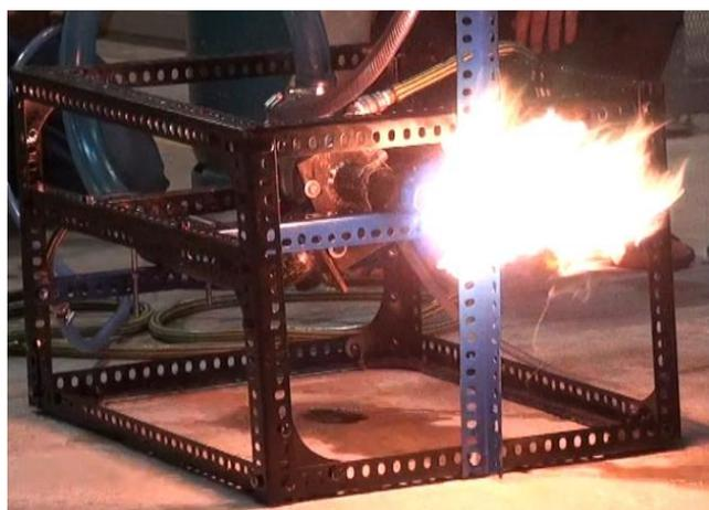
**Figure 4.4:** Unburned fuel burning at the exhaust
