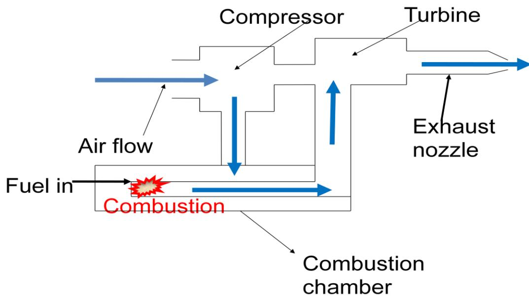
**Figure 3.2:** Overall design of the jet engine
