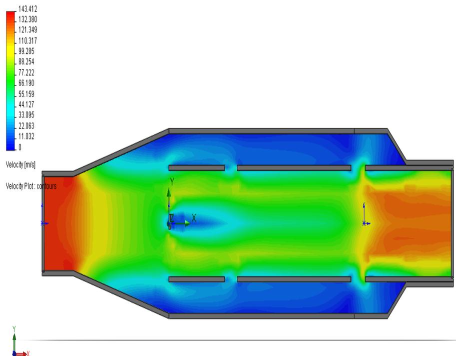
**Figure 4.1:** Velocity contour plot within the combustion chamber
