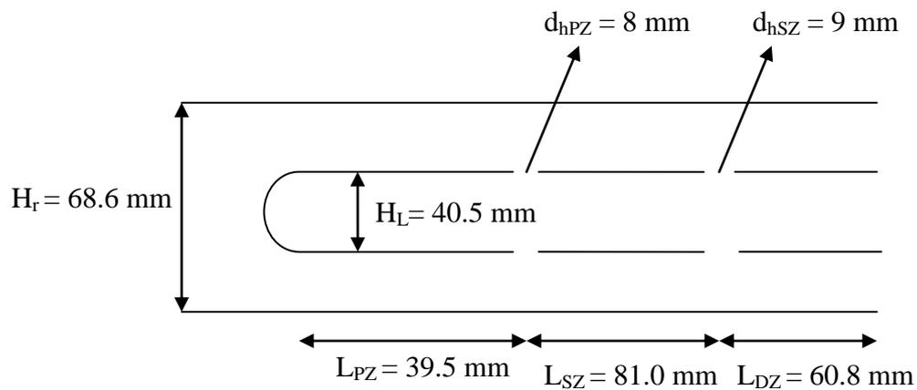
**Figure 3.5:** Dimension of the combustion chamber
