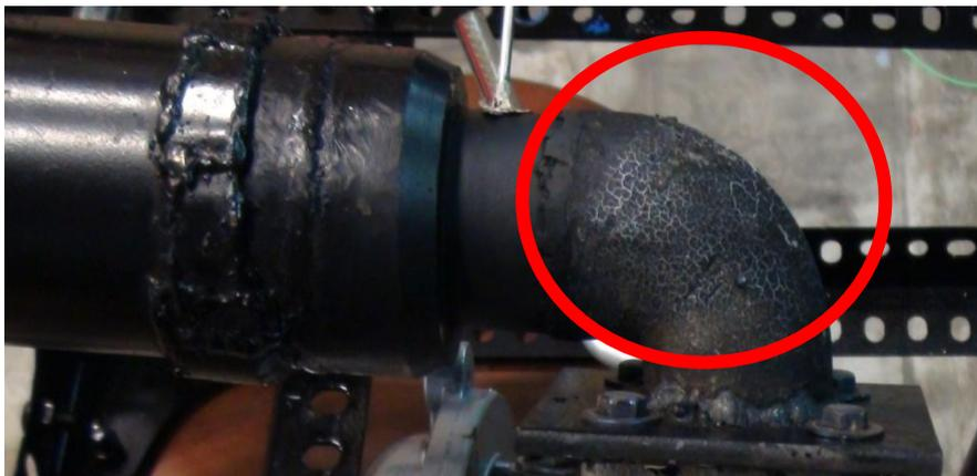
**Figure 4.15:** 90 degree pipe flange attached to the exit of the combustion chamber. The design is similar to the Whittle combustion chamber (Figure 4.15) where the exit of the combustion chamber is tuned more than  $90^\circ$
