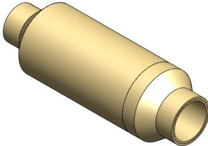
**Figure 3.6:** Isometric view of combustion chamber
