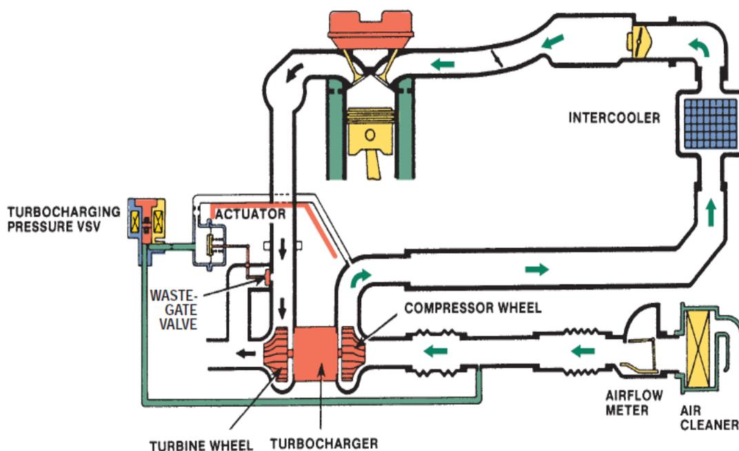
**Figure 2.7:** Exhaust gas and airflow of a typical turbocharger system
