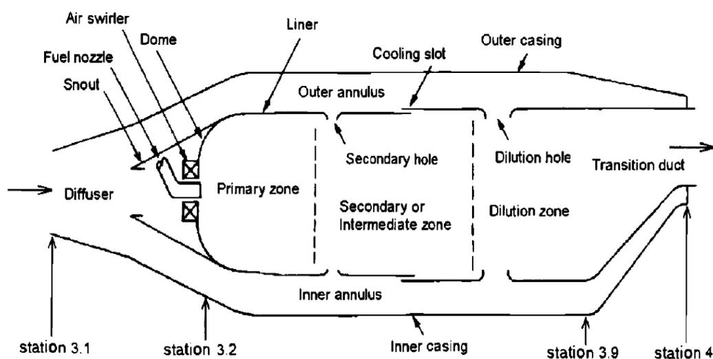
(a) Main features of the combustion chamber
