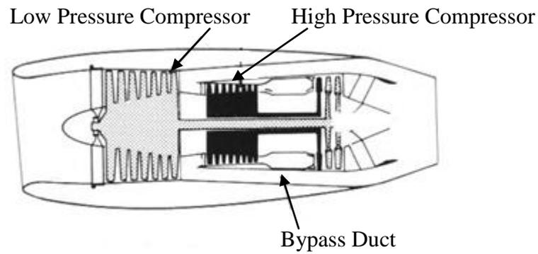
**Figure 2.3:** Schematic illustration of turbofan engine
