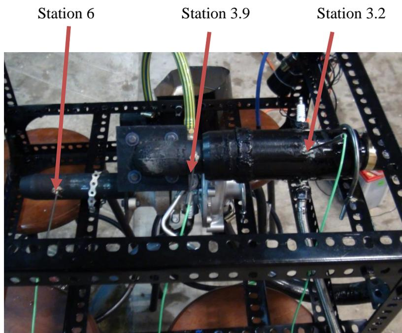
**Figure 3.18:** Thermocouple attached at different stations
