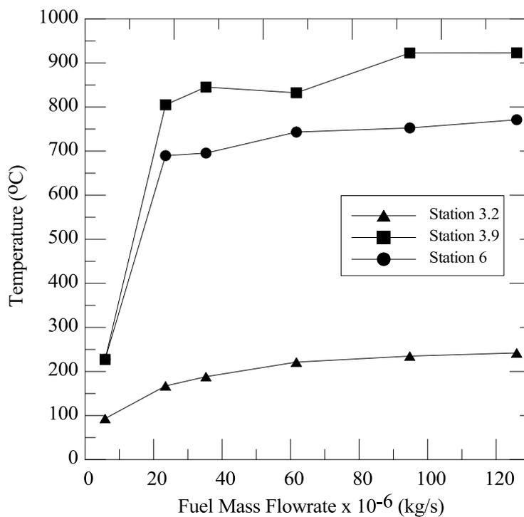
**Figure 4.12:** Graph of temperature mass flow rate at all three stations
