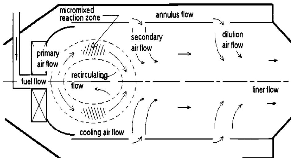
(b) Flow pattern of the combustion chamber
