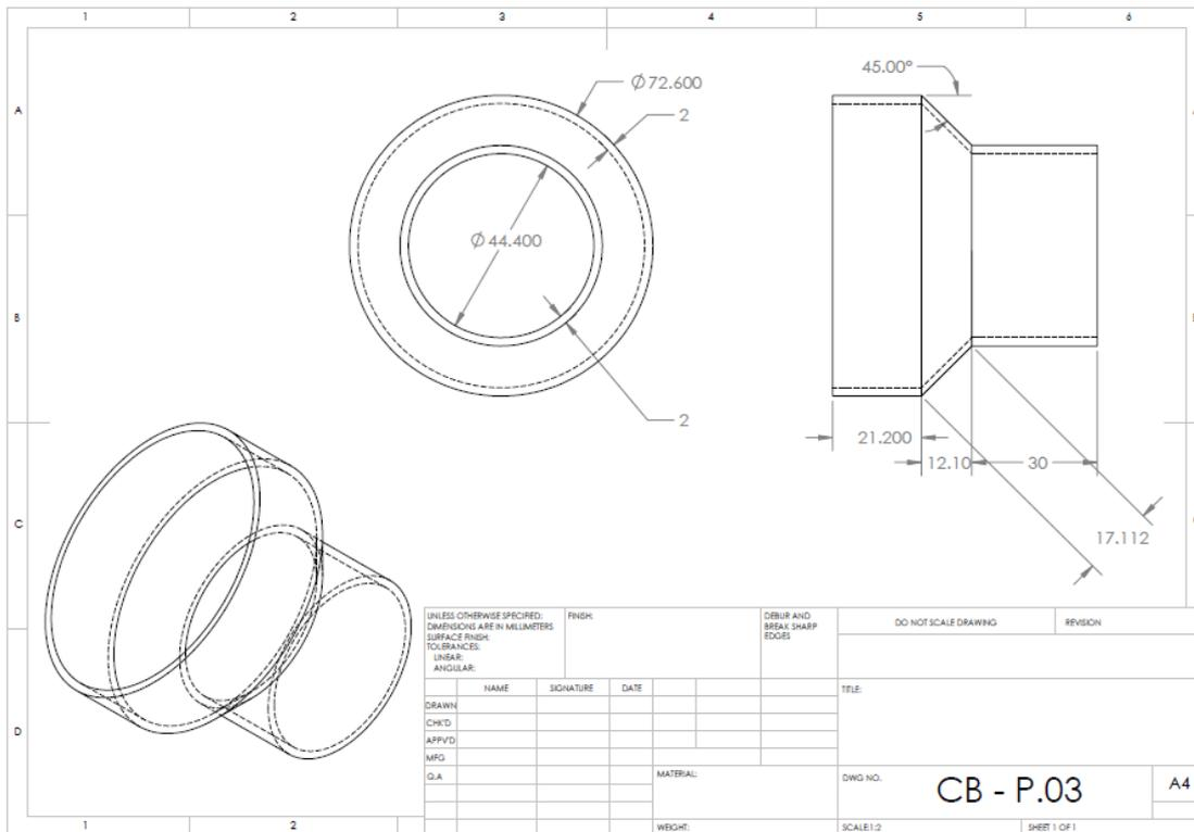
**Figure 6.3:** Two-dimensional drawing of liner holder
