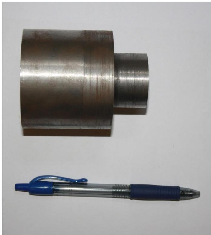
**Figure 3.10:** Side view of fabricated inlet diffuser
