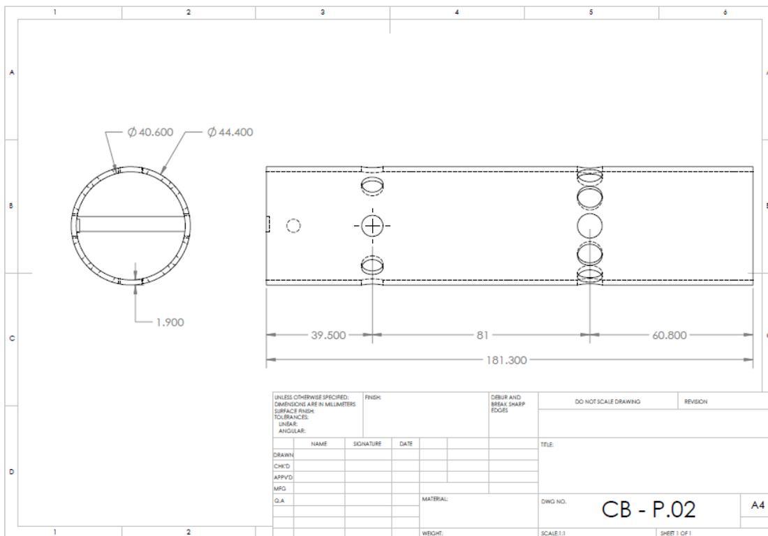
**Figure 6.2:** Two-dimensional drawing of inner liner
