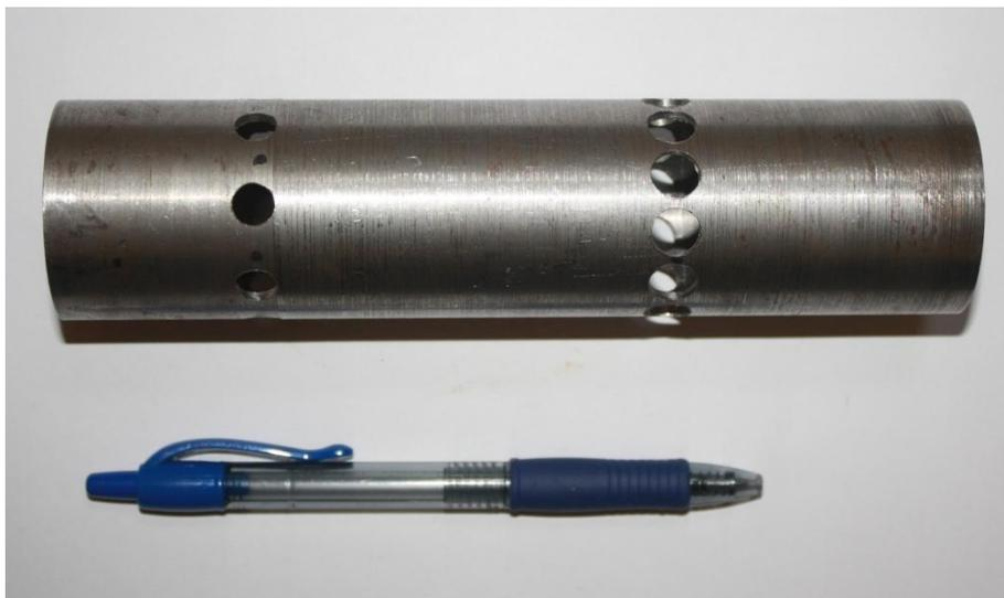
**Figure 3.11:** Side view of fabricated inner liner
