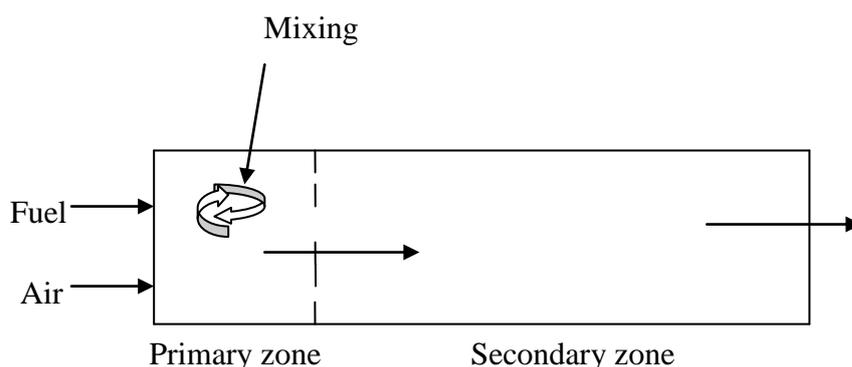
**Figure 2.9:** An idealized Bragg combustion chamber with a primary and secondary zone
