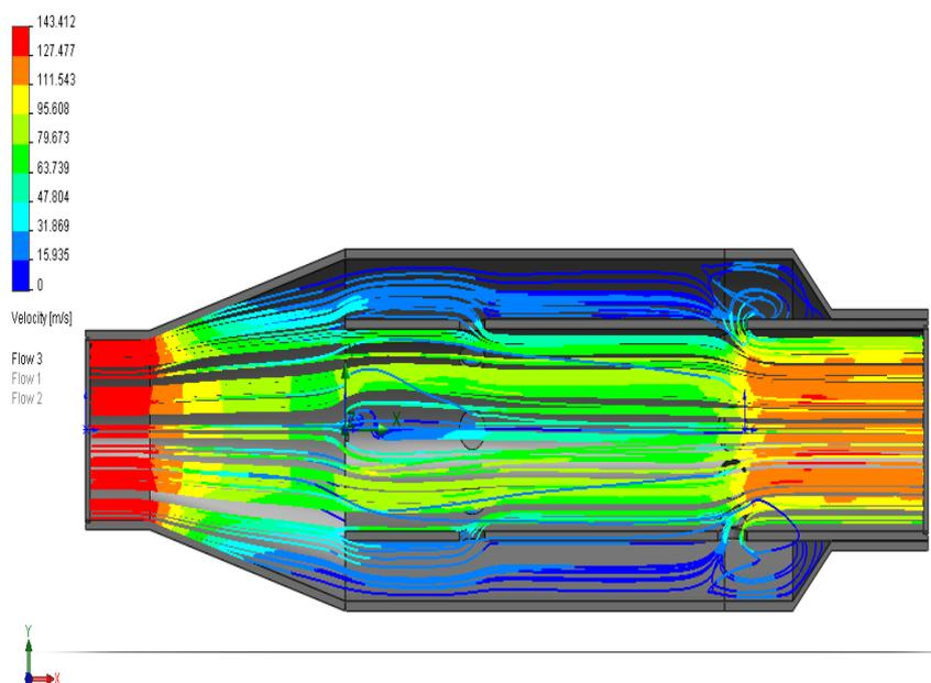
**Figure 4.2:** Velocity flow path of the combustion chamber
