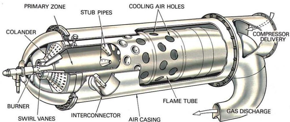
**Figure 4.16:** The Whittle combustion chamber
