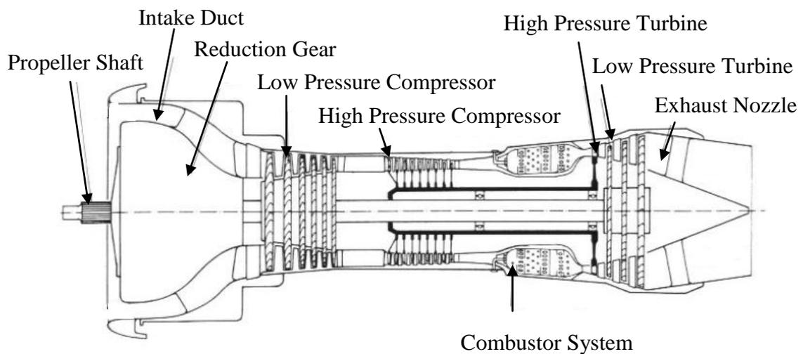
**Figure 2.4:** Schematic illustration of turboprop engine
