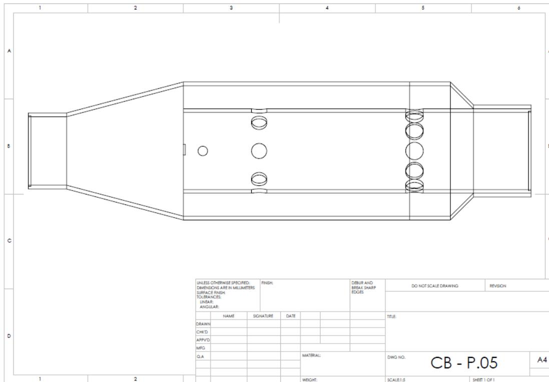
**Figure 6.5:** Two-dimensional drawing of completed assembled combustion chamber
