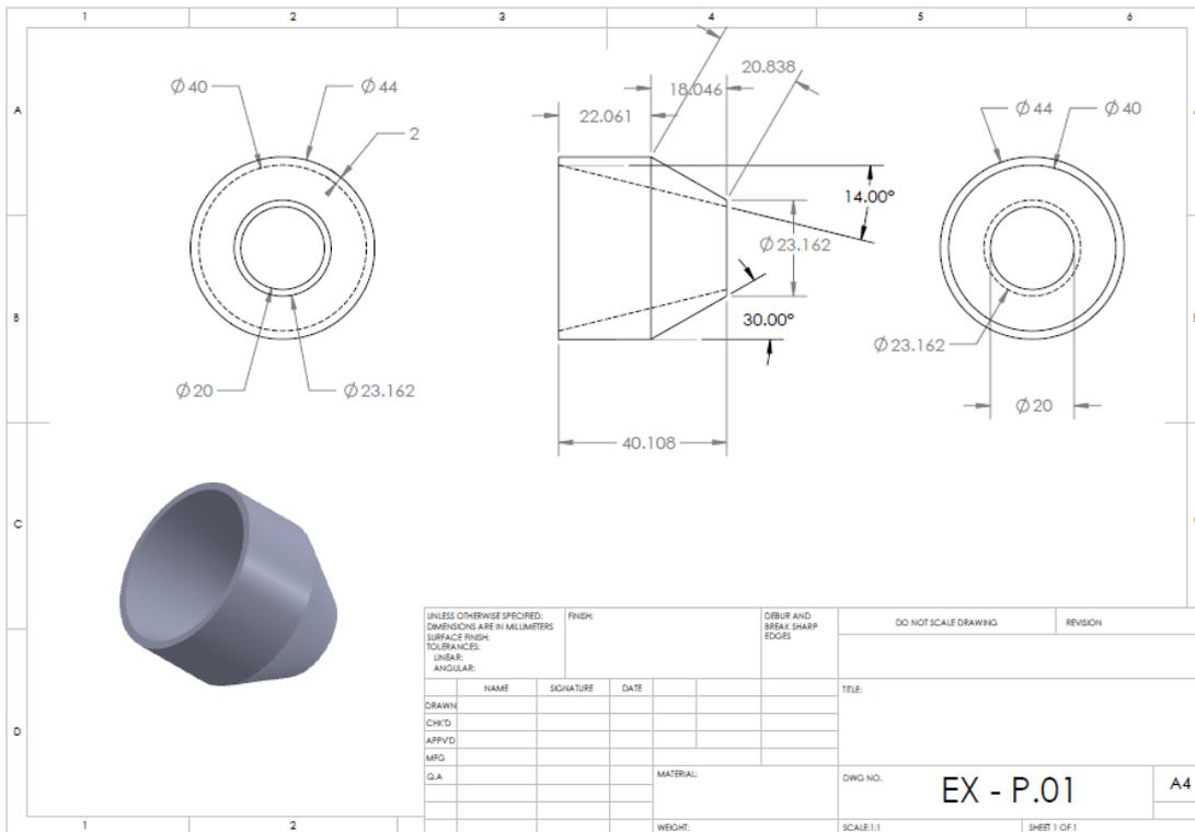
**Figure 6.6:** Two-dimensional drawings of nozzle
