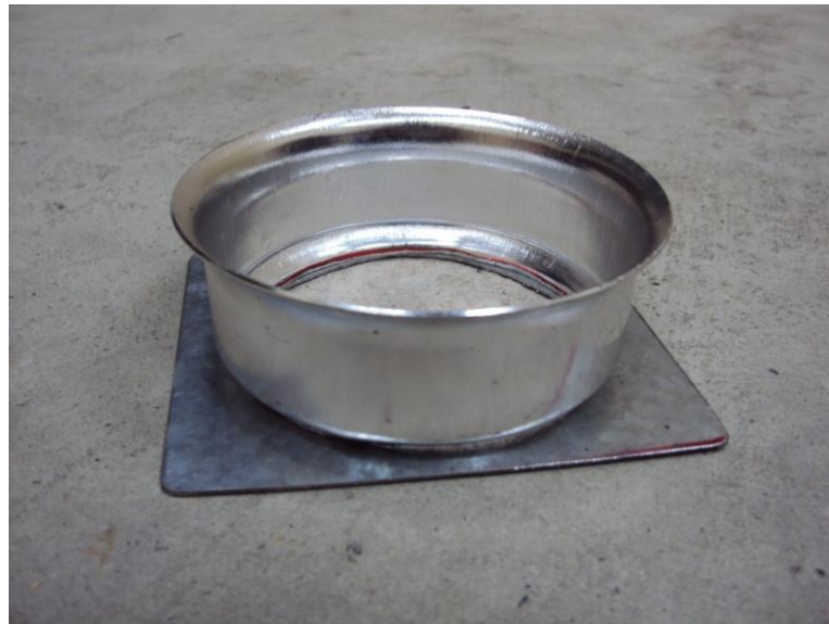
Figure 3.22: Fabricated bell mouth
