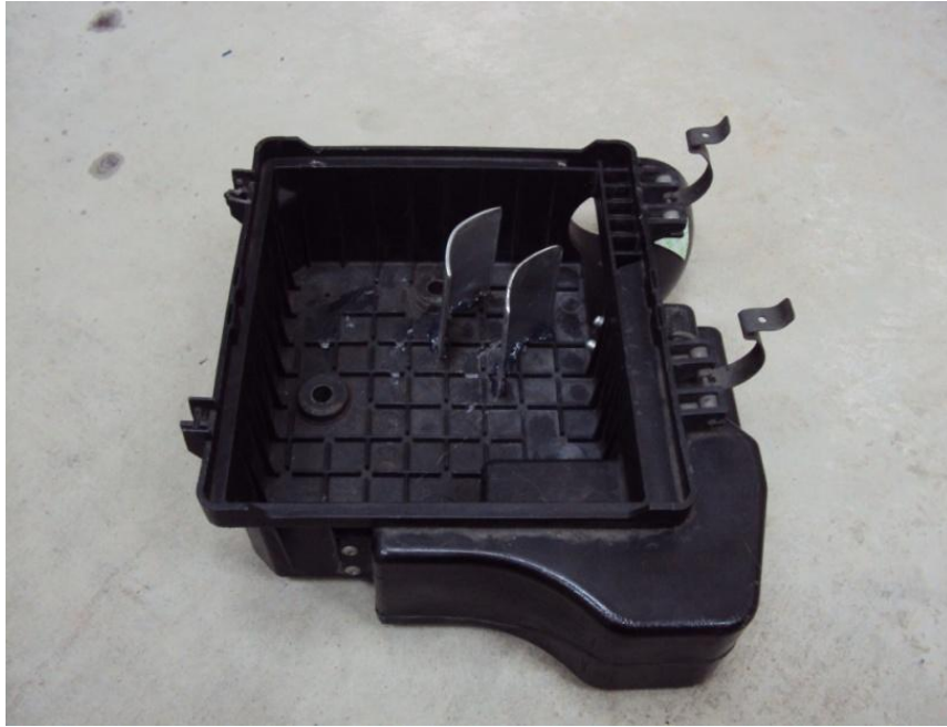
Figure 3.20: Guide vane installation on lower part of air box
