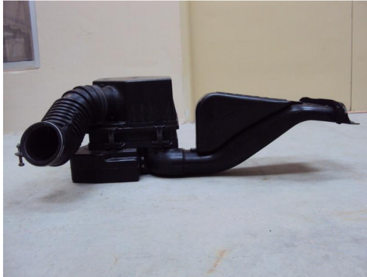
Figure 3.2: Proton Waja Air Box
