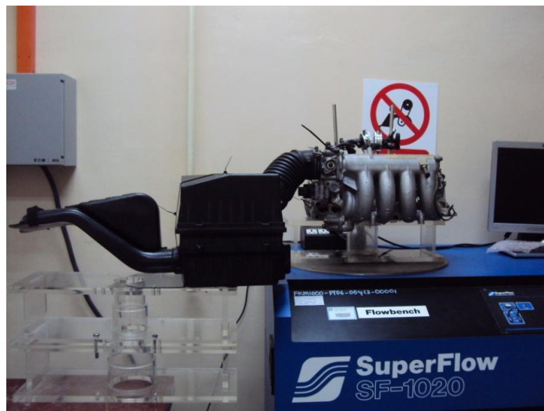
Figure 3.25: Air box setting on flow bench test
