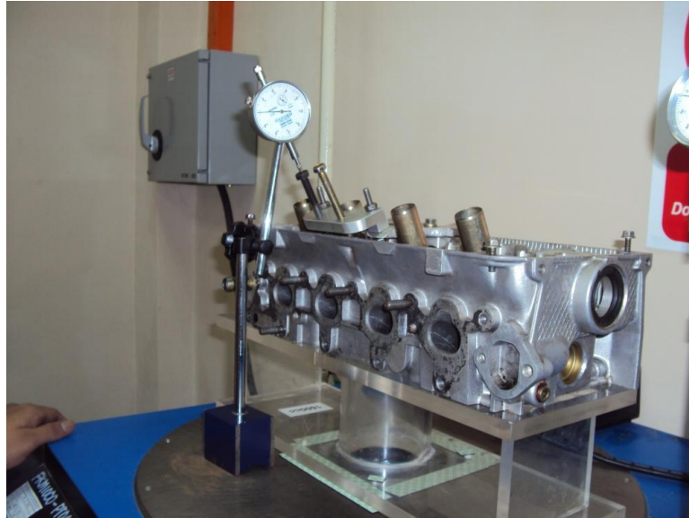
Figure 3.24: Cylinder head setting on head adapter on flow bench test
