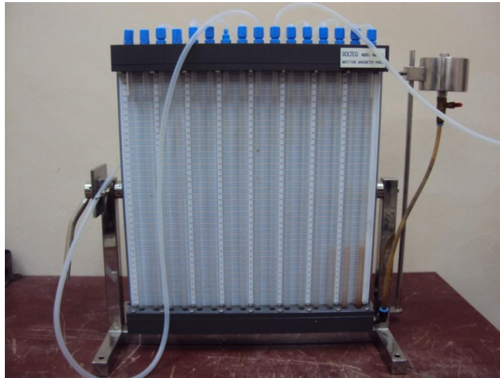
Figure 3.27: Multitube Manometer model SOLTEQ FM21-VT-A
