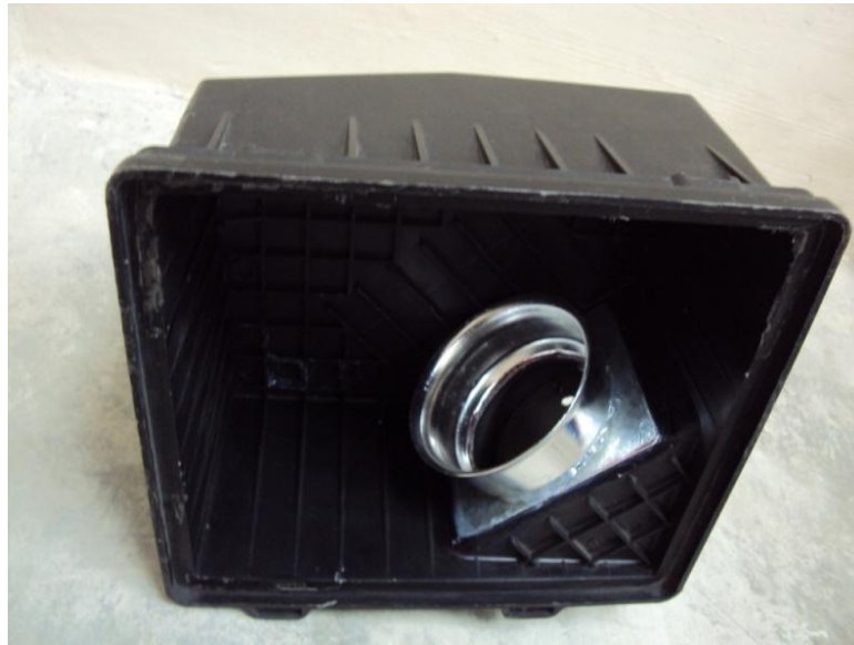
Figure 3.23: Fabricated bell mouth installation on upper part air box
