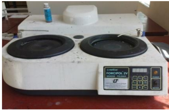
Figure 3.14: Polishing machine with PC diamond lubricant
