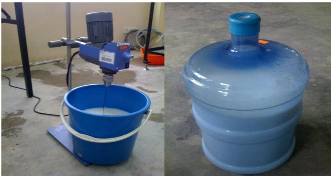
**Figure 3.4:** Stirring Process using Motorize Stirrer
