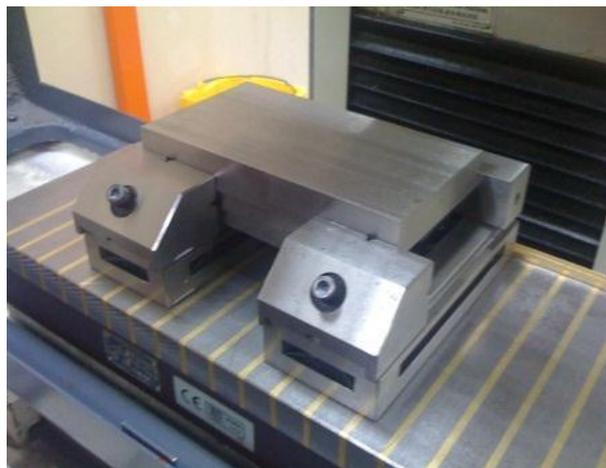
**Figure 3.7:** Work piece clamped using a steel clamp
