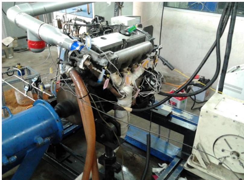
Figure 3.1: Diesel Engine Mitsubishi 4D68
