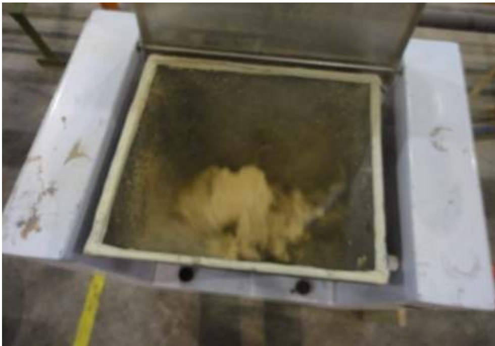
Figure 3.2: Wood fiber, nanoparticles and UF resin are mixing together
