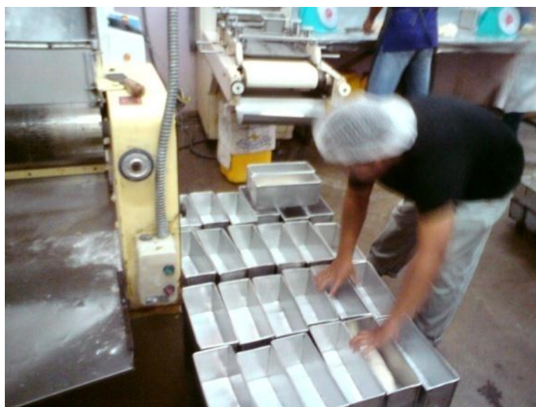
Figure 3.9: Place dough into baking tray
