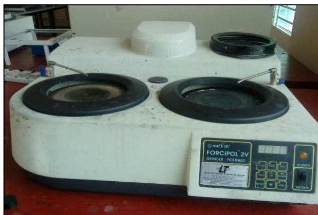
Figure 3.8: Polishing machine used for samples preparation
