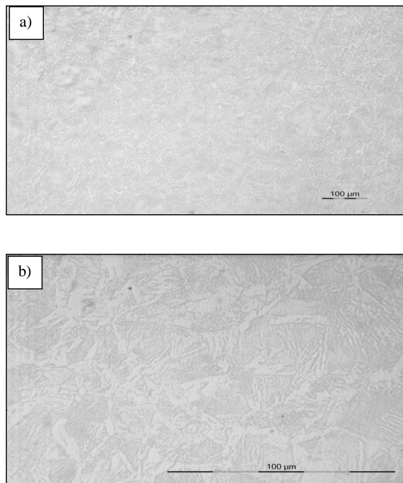
Figure 4.8: Microstructures of oil quenched of AISI 1070 steel at 980 °C: a) 100x magnification, b) 500x magnification
