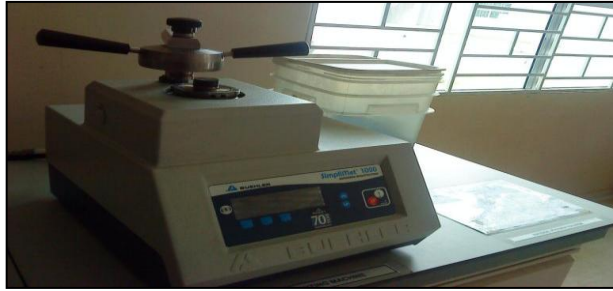
Figure 3.6: Hot mounting machine used for mounting all samples
