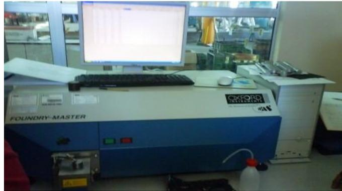
**Figure 3.5:** Spark emission spectrometer
