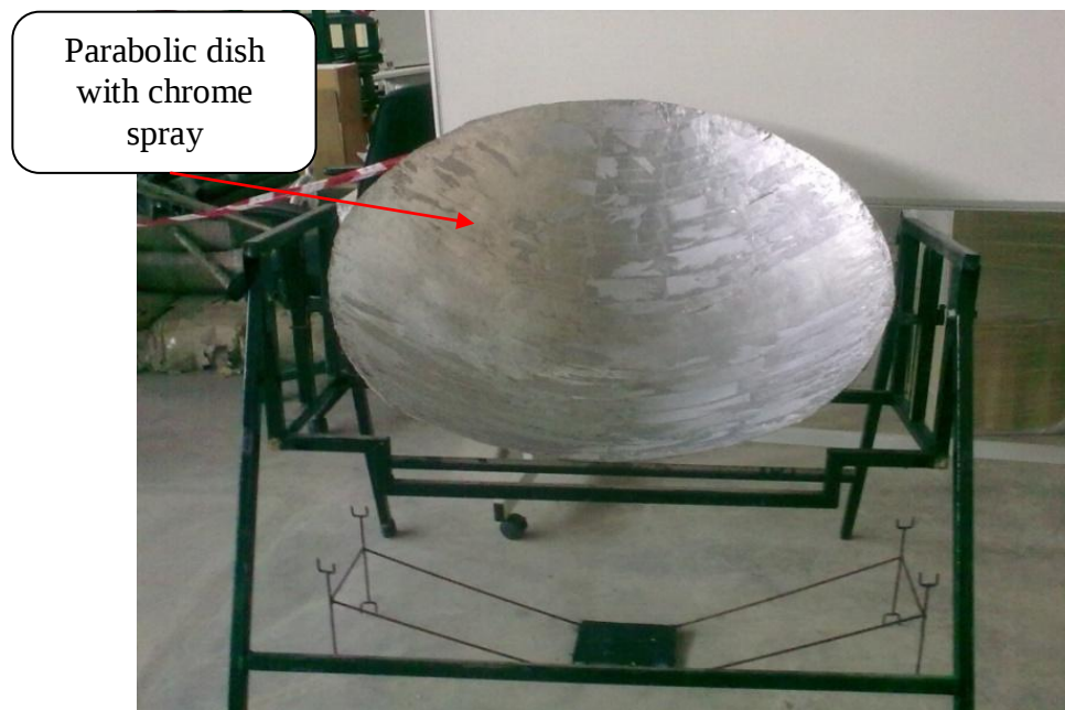
Figure 3.9: Parabolic dish with chrome spray
