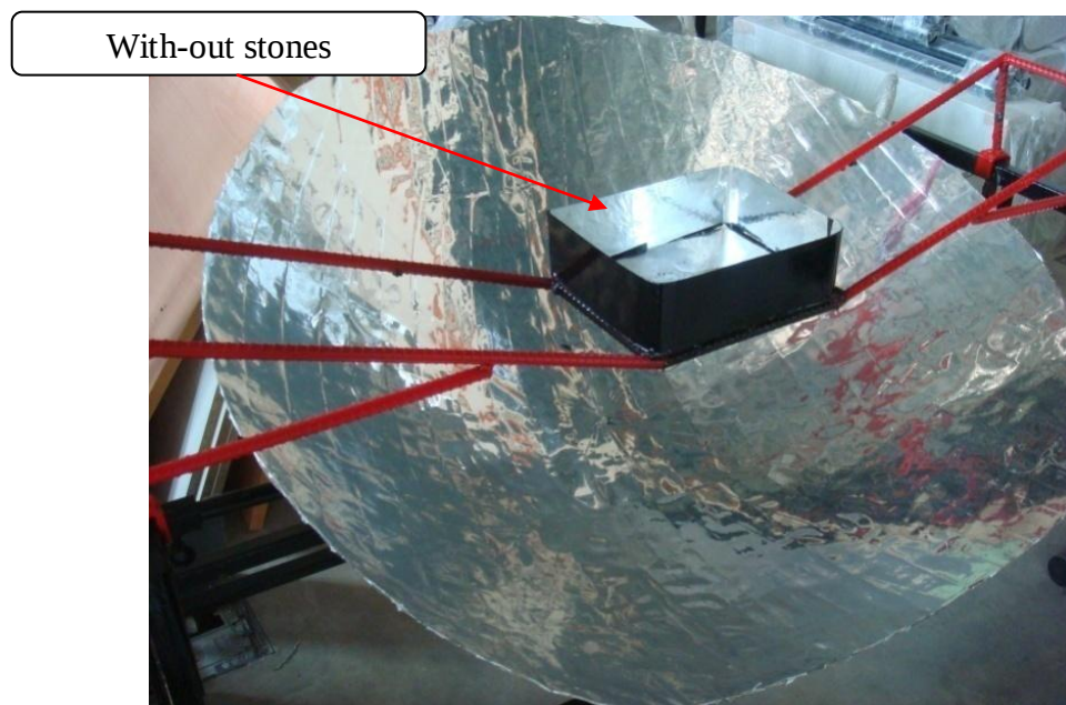
Figure 4.4: Experiment setting without thermal energy storage
