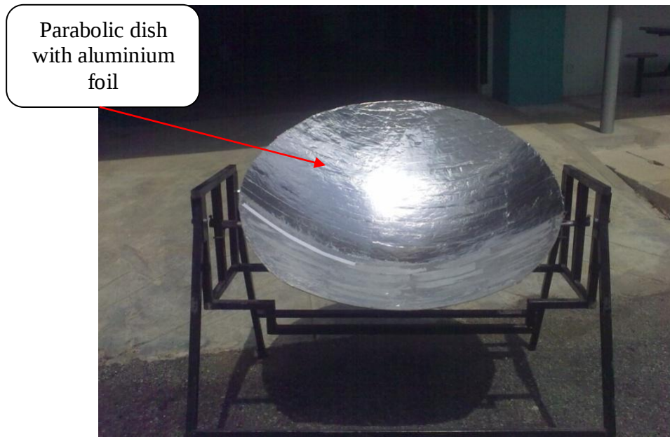
Figure 3.10: Parabolic dish with aluminium foil
