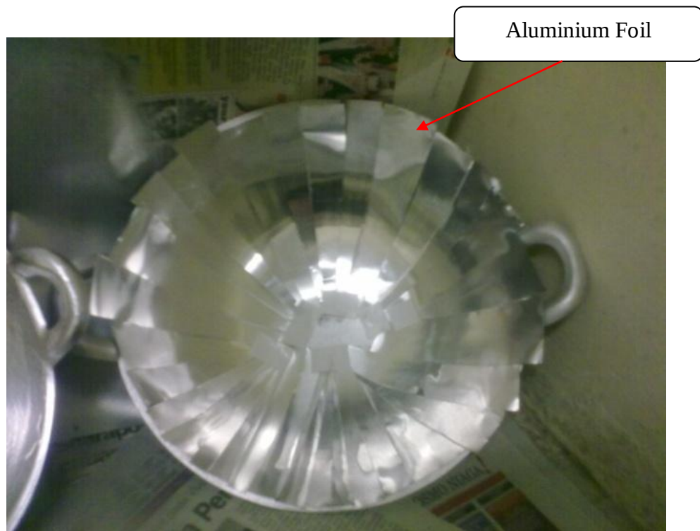
Figure 3.2: Aluminium foil reflector
