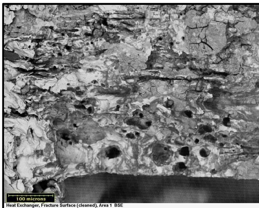
Figure 2.2 (b): Pitting corrosion in stainless steel backscattered SEM image
