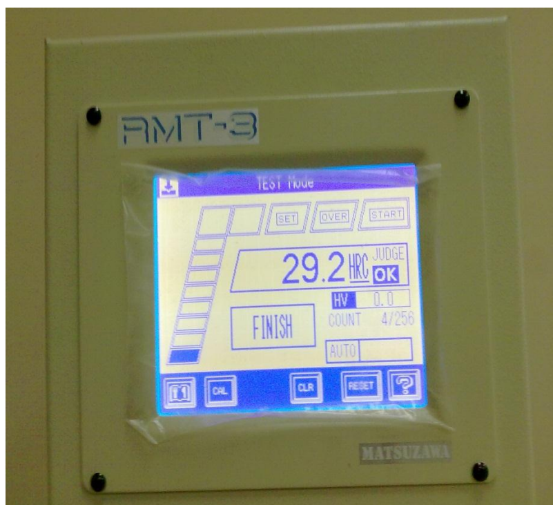
Figure 3.16: Result for HRC appears on screen after load applied.
