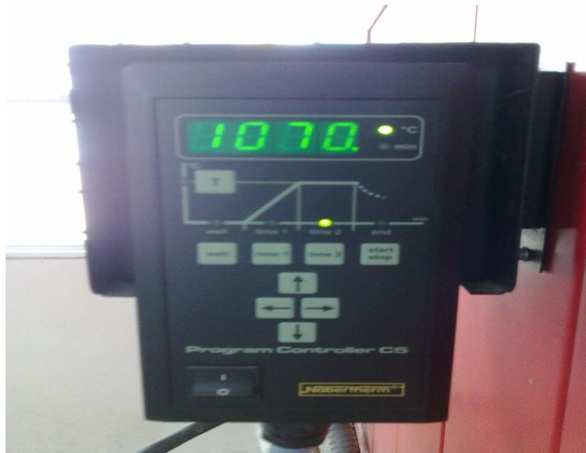
Figure 3.11: Program controller setting for furnace to heat and soaking specimens at 1070 °C
