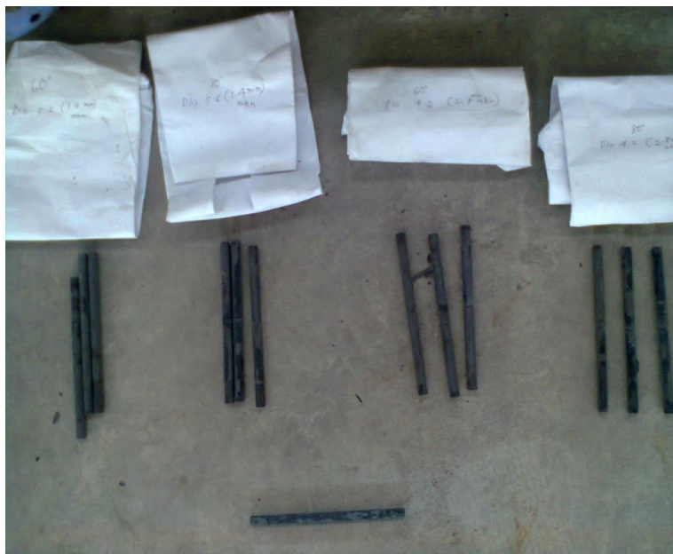
Figure 3.11: Specimens after full annealing
