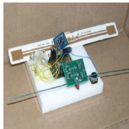
Figure 2.2.2 - Block diagram of the WISP (left) and photograph of a functioning Implementation (right).
