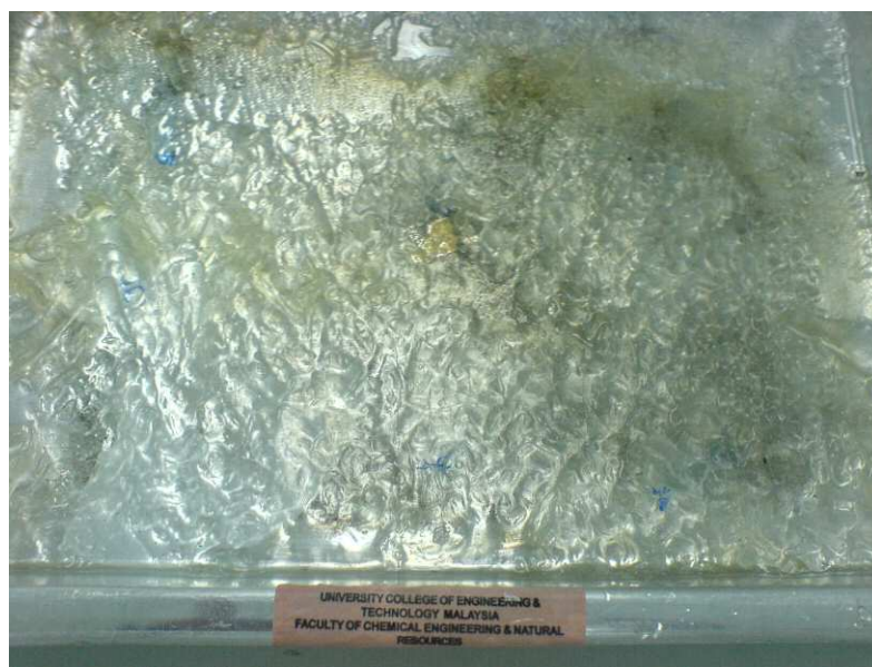
Figure 4.10: Over Heated Chitosan Membrane
