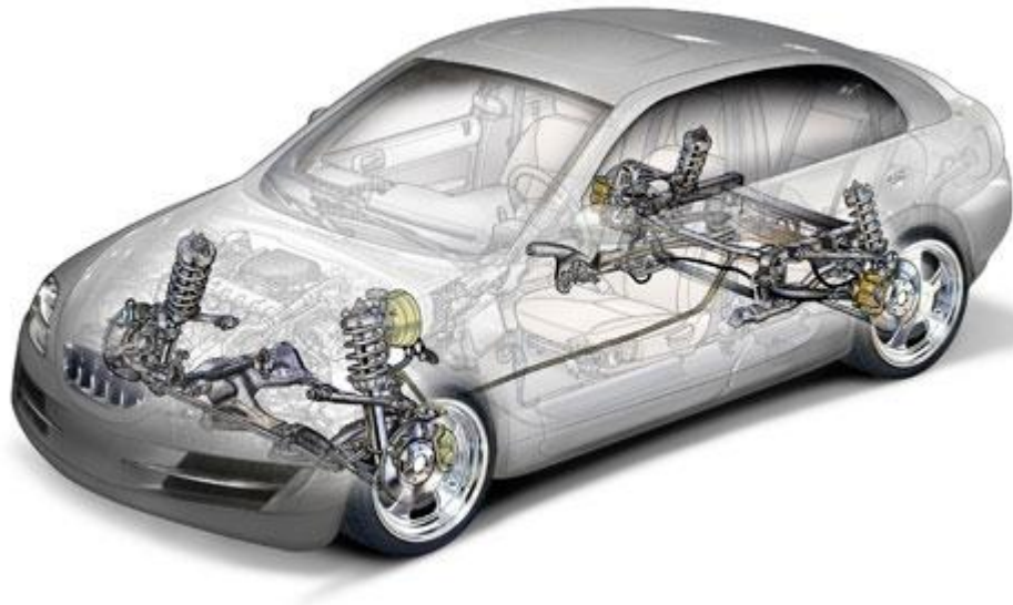
Figure 1.1: The location of car suspension system on a car
