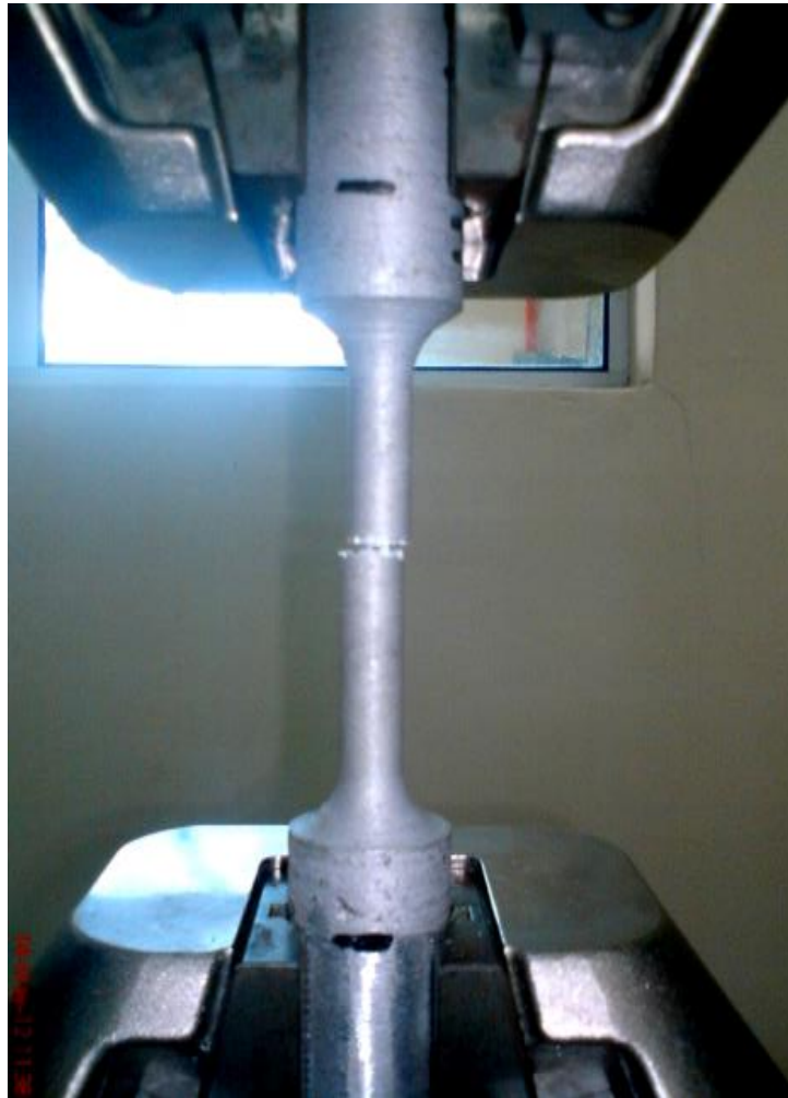
Figure 3.9: Specimen undergoes tensile test
