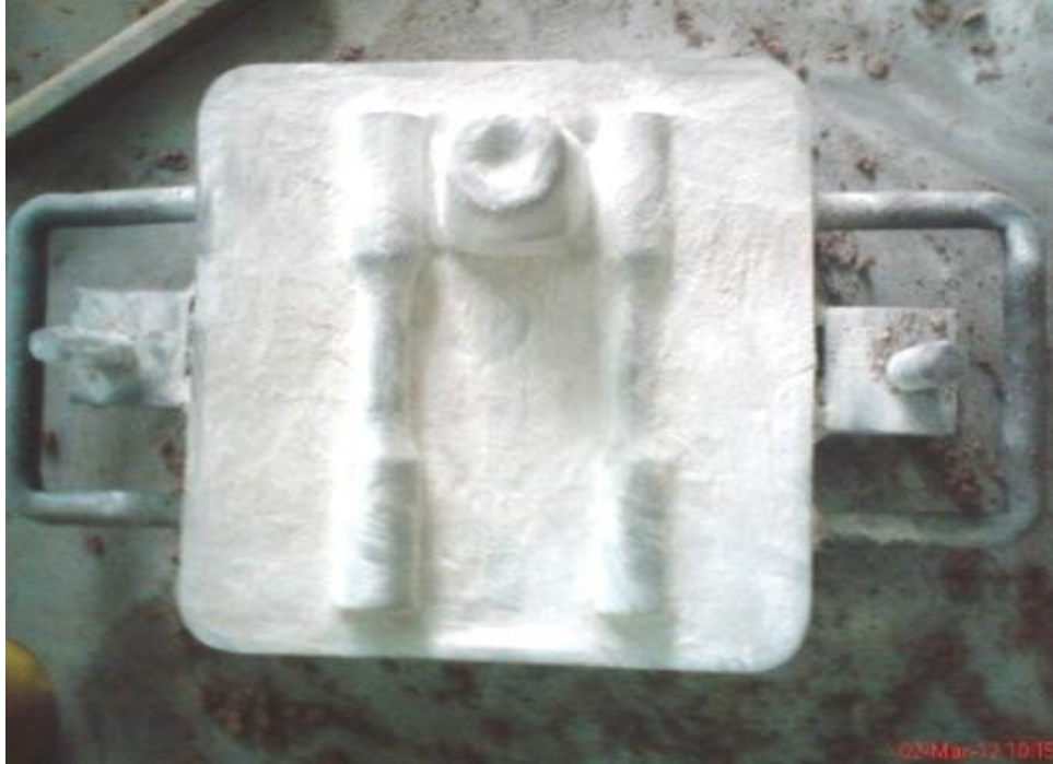
Figure 3.2: Sand mould making
