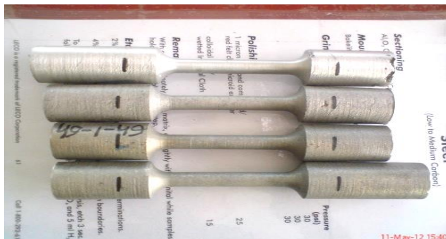
Figure 3.6: Specimen after machining process
