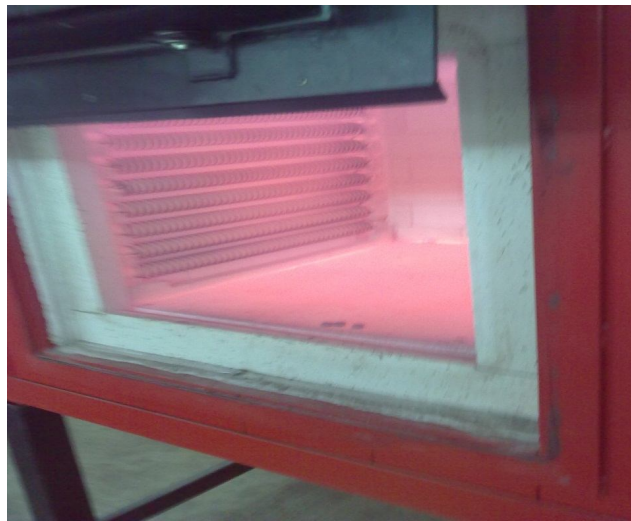
Figure 3.3: Furnace for pyrometallurgy process
