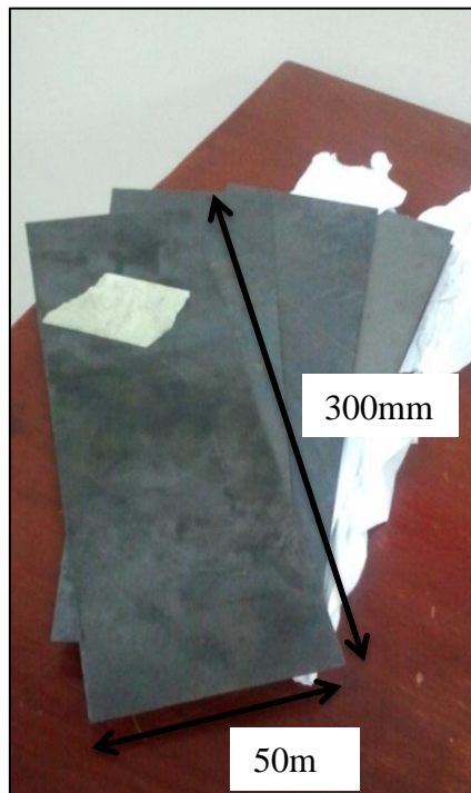
Figure 3.3 : Plates of Mild Steel AISI 1010 (300mm x 50 mm)
