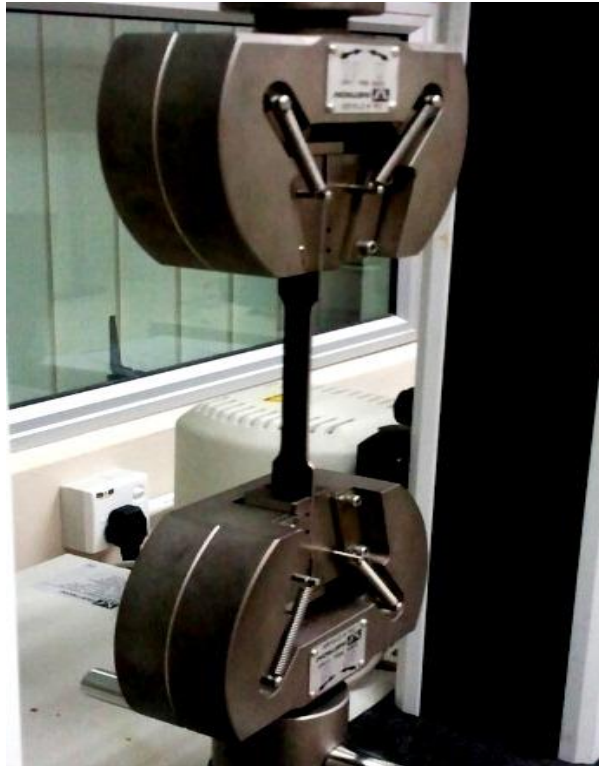
Figure 3.9 : Specimen attached in the tensile Machine during tensile test experiment.
