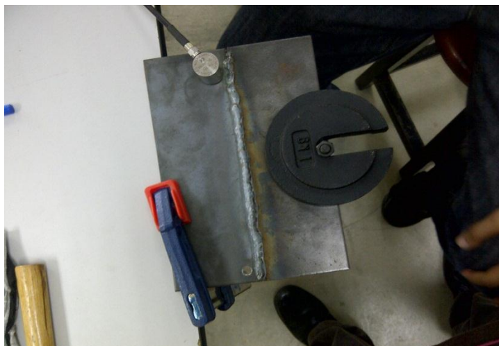
Figure 4.2: Experiment setup for defected welding joint
