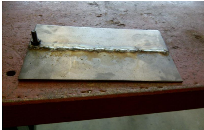
Figure 4.1: Defected welding joint
