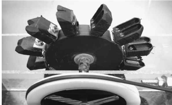
Figure 2.3: Details of the Pelton wheel showing the 12 vanes evenly spaced around the central hub.
