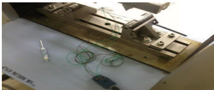
Figure 3.10: Strain gauge connected to data logger
