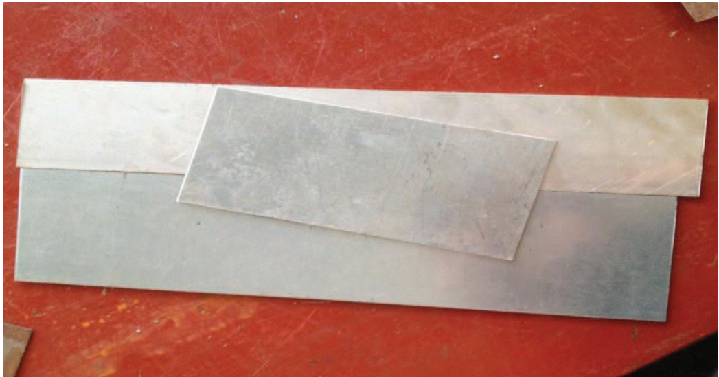
Figure 3.7: Plates of galvanized steel (220mm x 33 mm x 1mm)
