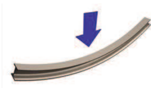
Figure 2.1: Bending of an I-beam
